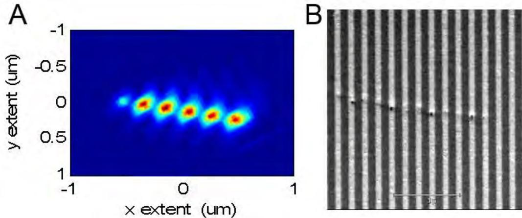
**FIGURE 8.** Suppression of line and space pattern while maintaining scratch signal detection. (A) Pattern-suppressed optical image of scratch defect; (B) SEM image of pattern and defect.
