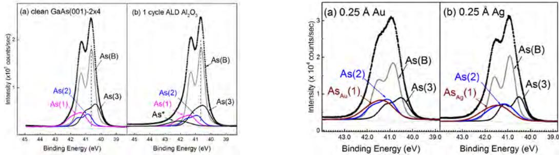
**FIGURE 1.** (Left) A fit to As 3d core-level spectra. (a) clean GaAs(001)-2x4 and (b) 1 cycle of ALD Al<sub>2</sub>O<sub>3</sub> on GaAs(001)-2x4. **FIGURE 2.** (Right) A fit to As 3d core-level spectra. (a) 0.25 Å of Au and (b) 0.25 Å of Ag on GaAs(001)-2x4.
