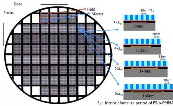
**FIGURE 2.** Line Space Block Copolymer arrays fabricated on a wafer with different focus-exposure conditions. The test areas contained sections (macros) with different guide structure pitches.[3]
