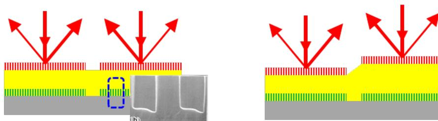
**FIGURE 1.** The left drawing shows the bottom grating asymmetry (BGA) caused by etch. The inset is only intended as an example to demonstrate an asymmetric grating and is taken from ref [4]. The right drawing schematically shows grating imbalance (GI)
