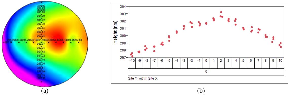
FIGURE 4. (a) Wafer map of height and (b) their value change on Y axis of wafer
