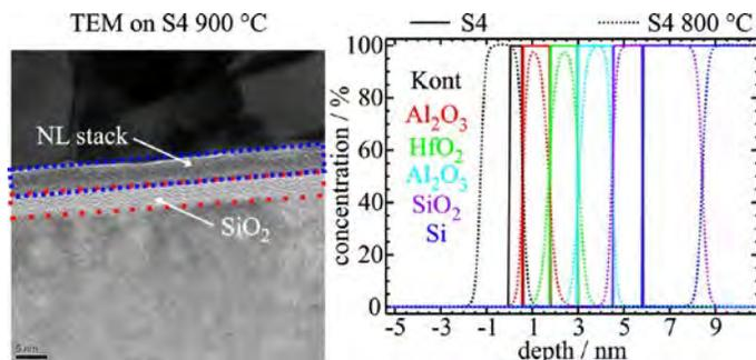
**FIGURE 3.** Comparison of the modeling results using the reference-free GIXRF-XRR of the as-deposited and the annealed sample S4. For comparison, also a TEM image is shown.
