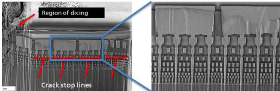
**FIGURE 1.** SEM cross-section images with crack stop structures of an Intel processor with 12 Cu metallization layers
