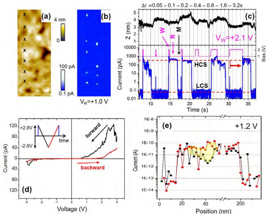
**FIGURE 1.** (a) constant-gap topograph (60x150 nm) and (b) corresponding current map at  $V_R$  after series of 14 voltage pulses. (c) time evolution of current (blue) and the gap (black) in response to voltage pulses (magenta) with WRITE (W), READ (R) and move (M) phases for positions marked by 'x'. (d) I-V spectrum with a hysteresis loop. Insert shows applied voltage vs. time. (e) Variation of HCS-LCS current difference at +1.2 V as a function of position for two traces.
