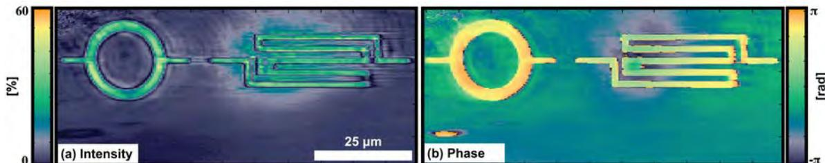
FIGURE 2. Reflection-mode Ptychography CDI intensity (a) and phase (b) images of 29nm tall nickel structures on a silicon substrate.
