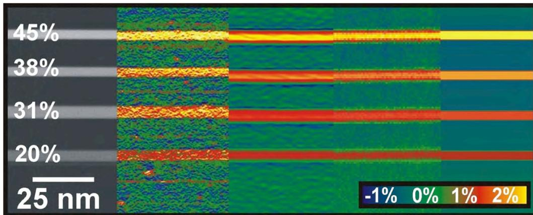
**FIGURE 2.** Shows a SiGe/Si test specimen with 10-nm-thick SiGe layers with different concentrations of Ge. Deformation maps for the growth direction showing the expansion of the lattice parameter relative to the unstrained substrate. The different maps from left to right have been acquired using geometrical phase analysis, dark field holography, precession electron diffraction and finite element simulations.
