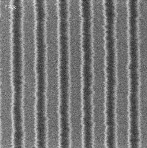
**FIGURE 1.** A typical top-down SEM image of line edges, recorded by J. Jussot from CNRS-LTM/CEA-LETI using a Hitachi CD-SEM. This image is recorded with a probe current of 6.0 pA at an acceleration voltage of 500 V. The number of integration frames is 16. The magnification is such that the field size is 2.76  $\mu\text{m}$  in length (1024 px) and 450-nm wide (1024 px). The resulting pixel size is approximately 2.7 nm  $\times$  0.44 nm.
