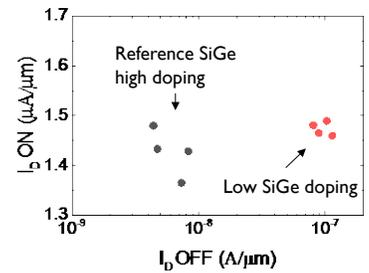
**FIGURE 12.** Impact of the SiGe SRB doping level (high vs low). In the low doping case, the formation of parasitic paths under the fin similar to the one presented here can induce a shift in the off-state leakage of the transistor.
