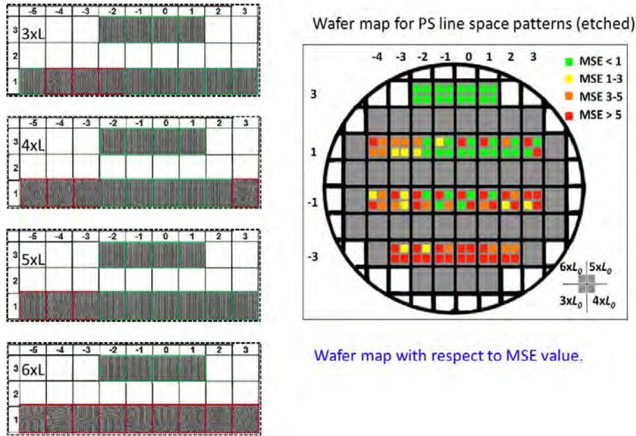
**FIGURE 3.** CD SEM images and results of optical model fitting for Line Space Block Copolymer arrays fabricated on a wafer with different focus-exposure conditions..[3]
