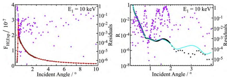
**FIGURE 2.** Results of the reference-free GIXRF-XRR (solid lines) for sample S5 ( $\text{Al}_2\text{O}_3 / \text{HfO}_2 / \text{Al}_2\text{O}_3$  layer sequence) in comparison to the experimental data (black dots). The residuals are also plotted as violet dots.
