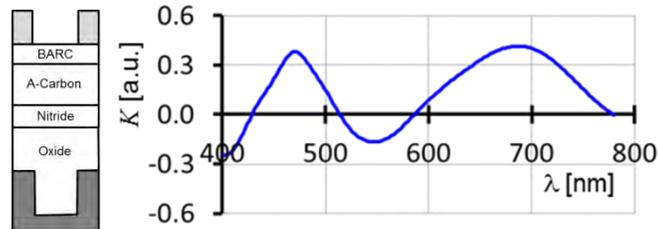
FIGURE 2. Simulated example of a swing curve
