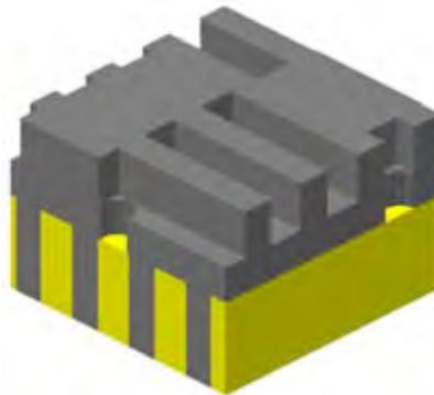
**FIGURE 3.** Simulation model of silicon dioxide (gray) over tungsten (yellow).
