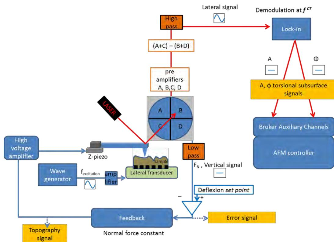
FIGURE 1. Schematic of the subsurface torsional imaging using scanning probe microscope.
