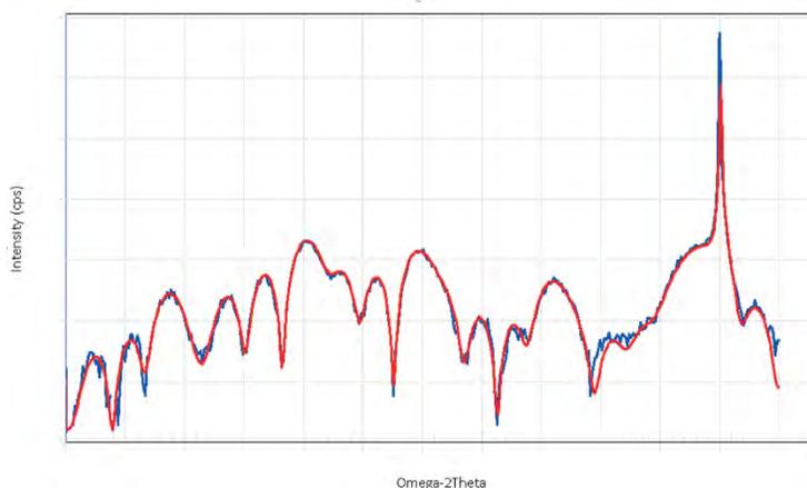
**FIGURE 1.** HRXRD  $\omega$ - $2\theta$  scans around the symmetric (004) Bragg reflection from a SiGe/Si nanosheet on a bulk Si substrate. Analysis of the diffracted intensity distribution gives information on the lattice parameter of the individual layers with respect to the silicon substrate. Ge concentration and layer thickness are calculated from the best fit simulations (red) of the measured (blue) intensity profiles.
