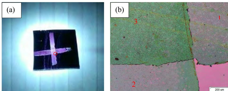
**FIGURE 1.** (a) Image of the cross-patterned 2-mm wide graphene stripes and (b) enlarged optical image of the red circle at the lower-right corner of the graphene cross in (a).
