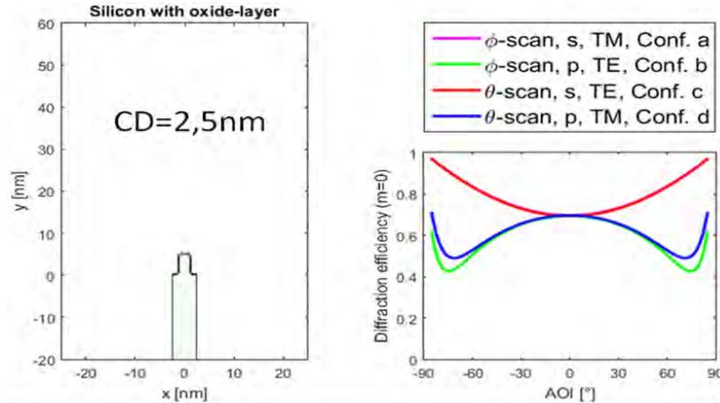
**FIGURE 2.** Numerical simulation of reflectance curves for a Si grating, period = structure height = 5 nm, CD = 2.5 nm
