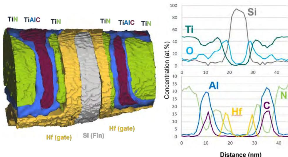
**FIGURE 3.** (left) Atom probe analysis of a 14-nm finFET device along the gate direction. Iso-concentration surfaces of arbitrary value were chosen, rather than the individual ion points, to clearly demarcate the various layers within this highly engineered structure. (right) Concentration profile of the central sub-volume of the device (gate-fin-gate). The accuracy of the measured compositions is affected by the relative field differences of neighboring layers.
