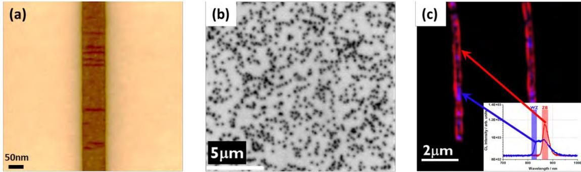
**FIGURE 3.** (a) AFM on InP fins after defect etching revealing stacking faults emerging at the fin surface. (b) CL map on blanket GaN layer. Threading dislocations act as non-radiative recombination centers and hence appear as dark spots. (b) CL map on InP fins. The relaxation of InP grown on Si is facilitated by the formation of a dense network of twinning planes leading to a Wurtzite crystal structure detectable by CL.
