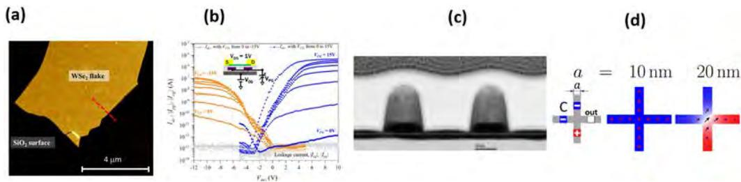
**FIGURE 3.** (a) WSe<sub>2</sub> flake of 7.5nm teck. (b) n & p bi-polarity of WSe<sub>2</sub> controlled by gate can be applied to enable new ambipolar logic XOR gates (c) XTEM of magnetic tunnel junctions on a MgO free layer for a Spin-Torque majority gate (STMG) (d) Micro-magnetic simulations of the domain switching of the 3-input STMG as a function of dimension. Sources: (a) & (b) Ref. 5, (c) and (d) from Refs. 6 and 7, respectively.
