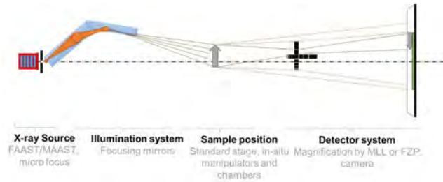
**FIGURE 4.** Scheme of a nano XCT setup for advanced packaging metrology, using novel X-ray sources and optics.
