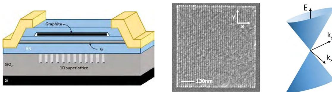
**FIGURE 2.** **Left:** schematic of electrostatic gating through a 1D superlattice. The top gate modulates the carrier density while the lower tunes the superlattice strength. **Center:** 20nm full-pitch superlattice of thin HSQ on top of SiO<sub>2</sub>. **Right:** highly squeezed Dirac cone demonstrating the anisotropic transport resulting from the 1D superlattice.
