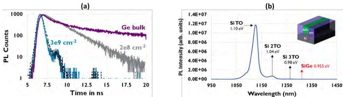
**FIGURE 2.** (a) Photoluminescence decay measured on thick relaxed Ge layers with different threading dislocation densities at 77K. (b) PL spectrum (77K) of an array of relaxed  $\text{Si}_{0.3}\text{Ge}_{0.7}$  fins (225nm wide) selectively grown in a STI matrix.
