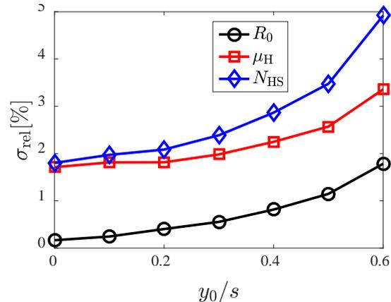
**FIGURE 3.** Relative standard deviation for  $R_0$ ,  $\mu_H$  and  $N_{HS}$  vs. distance to the edge,  $y_0$ , for  $w = 3.5s$  and  $L=7s$ . The probe should not be placed further from the edge than  $y_0 = 0.4s$ , which is the standard today, since a larger distance will lead to lower precision. Higher precision can be achieved by moving the probe pins closer to the boundary.
