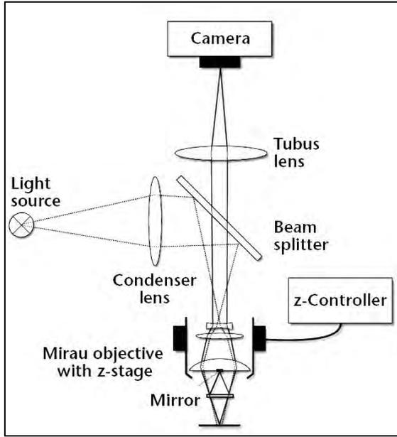
**FIGURE 1.** Optical path in white-light interference microscopy. (figure attributed to Polytec GmbH)
