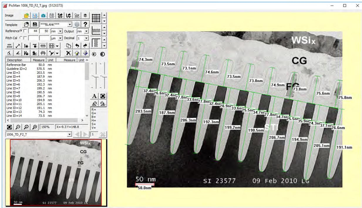
FIGURE 1. Dimension measurement example from a TEM image. [1]
