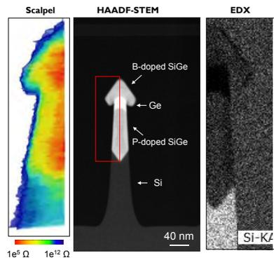
**FIGURE 7.** Site-specific structural, chemical and electrical information. The same device can be studied by Scalpel SPM and TEM. In this case, the chemical sensitivity of EDX is combined to the carrier profile capability of SSRM and the structural analysis of TEM in the red rectangle
