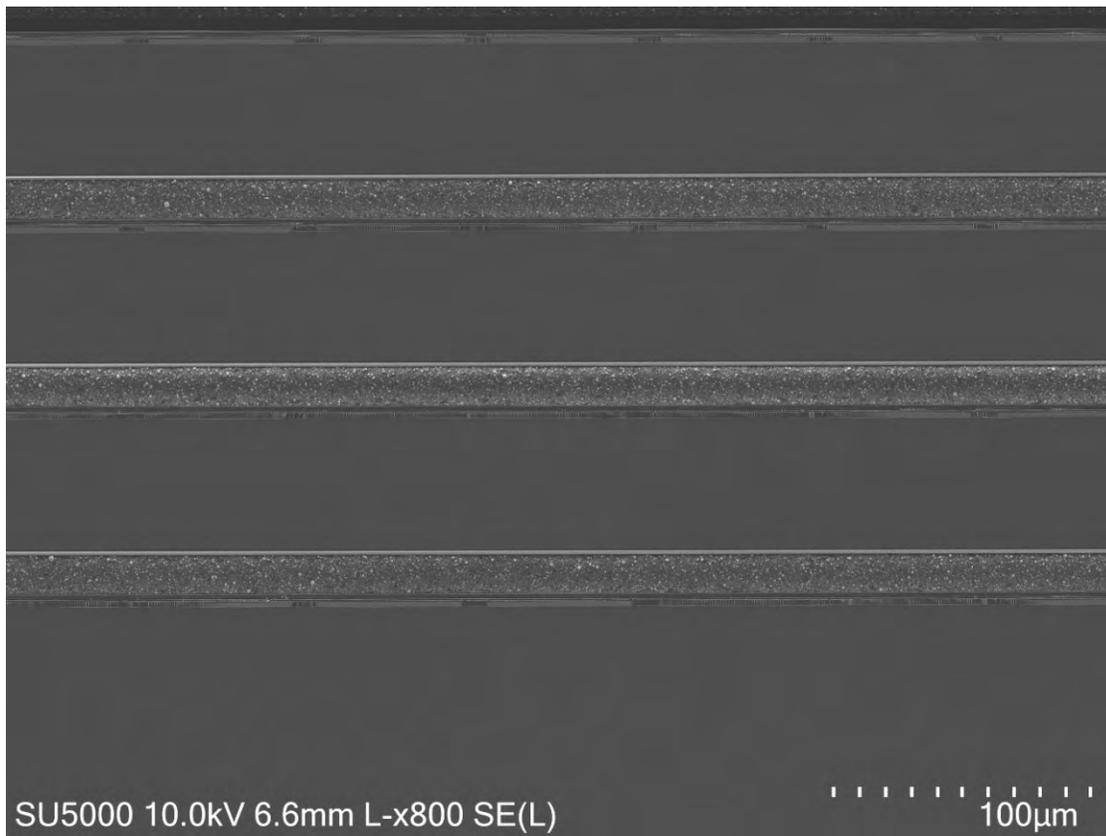
**FIGURE 1.** SEM Image of Cross Section of stacked chips prepared with a pico-second laser tool and Broad Argon ion Beam Tool
