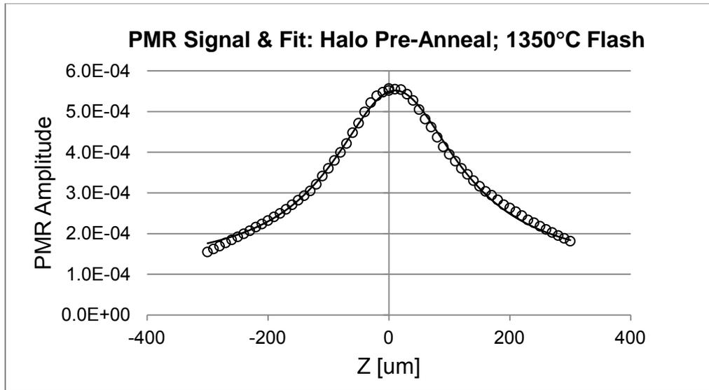
FIGURE 1. Exemplary PMR signal and fit for sample w/o PAI as a function of pump focal plane from sample surface.
