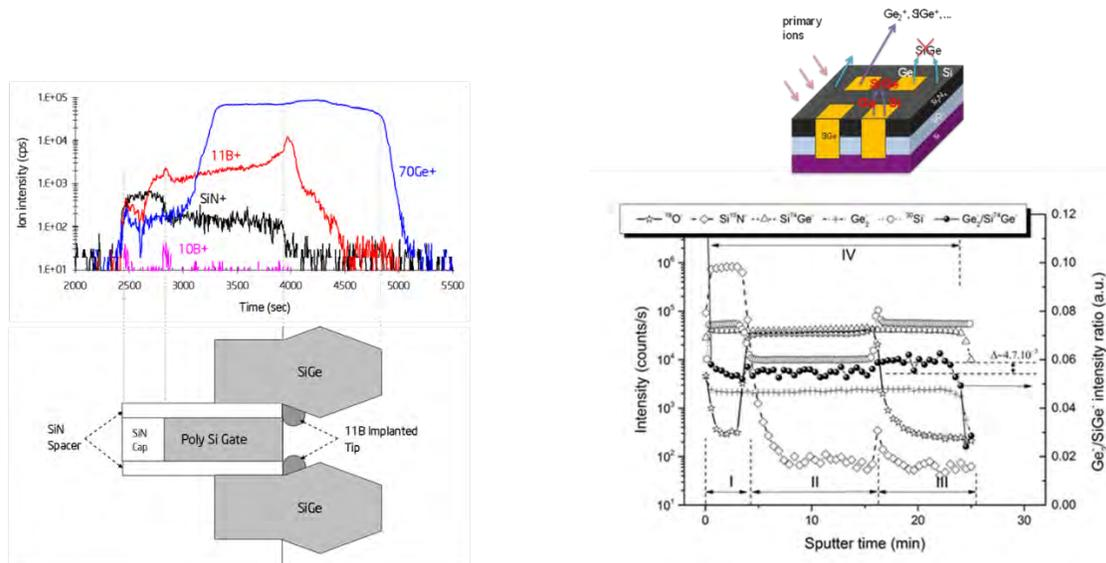
**FIGURE 2.** SIMS methods under development for measuring nanoscale device material parameters. 1.5D SIMS on left and Self-Focusing SIMS on the right [6].
