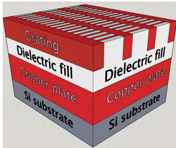
**FIGURE 4.** Copper Cross-Grating Structure showing a copper plate below the top cross-grating.[5, 6]
