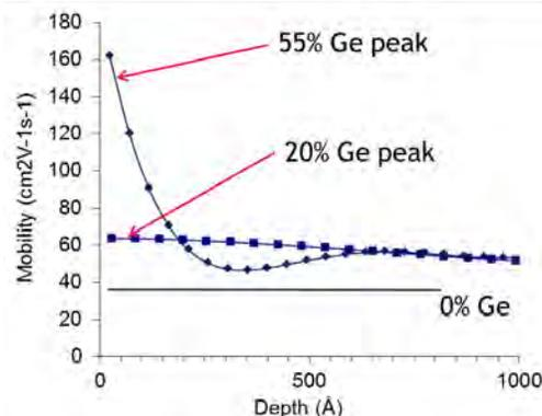
**FIGURE 2.** ALPro showed 70% increase in mobility for 20% Ge sample and 4.3x increase for 55% Ge sample. 55% Ge sample concentration peak was at  $\sim 20 \text{ \AA}$  (confirmed by AR-XPS)[6].
