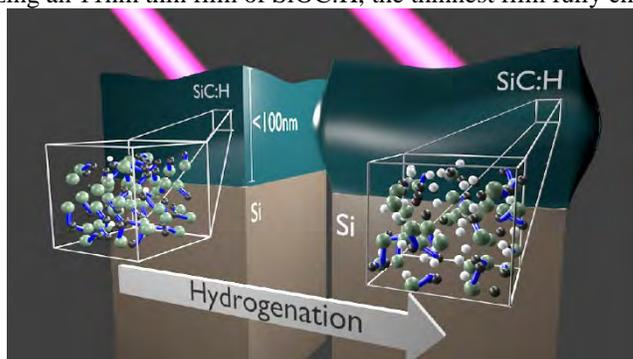
**FIGURE 1.** Artist's illustration of Coherent EUV Nanometrology. This study revealed increasing hydrogenation decreased average bond coordination and decreased compressibility in low- $k$  SiC:H thin films<sup>2</sup>.
