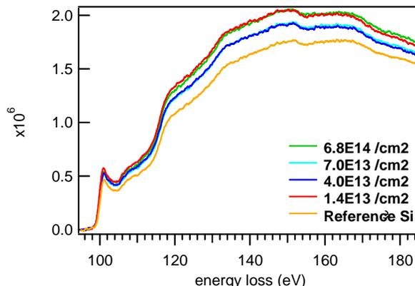
FIGURE 3. ELNES spectra from Si-sub. at different doses at 100 nm depth from the Si-sub. surface.
