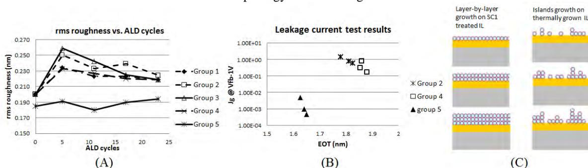
**FIGURE 3.** (A) rms roughness of the ALD  $\text{HfO}_2$  grown on the ILs; (B) MOS capacitor leakage current ( $J_g$ ) and EOT test data from 23 cycles of  $\text{HfO}_2$  deposition on different types of ILs; (C) Growth model of ALD  $\text{HfO}_2$  on different ILs
