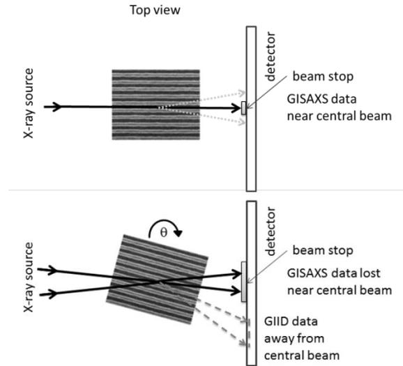
**FIGURE 2.** Top view of GISAXS vs. Grazing Incidence In-Plane Diffraction (GIID) configuration. On the left, GISAXS requires a collimated beam and fine alignment of features along the beam direction. A beam stop is used to prevent the detector from saturating in order to measure scattering. On right, rotating sample in-plane creates conditions for reflection from multiple GIID scattering sites in the sample. GIID can use a focused beam to significantly increase intensity on the sample.
