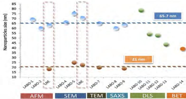
**FIGURE 1.** Measurements of nanoparticle size as a function of techniques used at different laboratories. Courtesy of Club Nanométrie.
