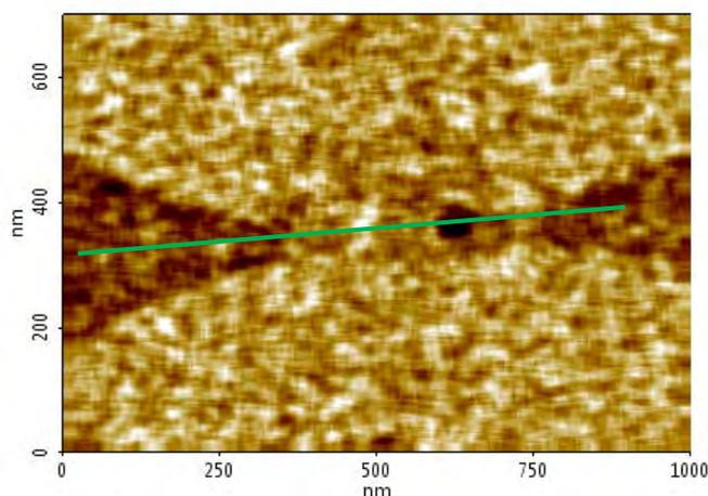
**FIGURE 6.** An SCM capacitance image of the region containing Device 6's sensor-drain interface, vacuum-channel, and insulated gates. Brighter colors correspond to relatively more positively charged areas on the device whereas darker colors correspond to relatively more negatively charged areas. Note the absence of electrical evidence for a functioning second
