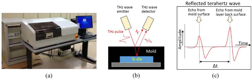
**FIGURE 1.** (a) TS9000 measurement unit (left side on the table), rack mounted controller electronics and optics (right), and controller PC (right side on the table). (b) Measurement configuration of overlaid mold thickness with pulsed THz radiation. (c) Example of reflected time-domain waveform from the DUT.
