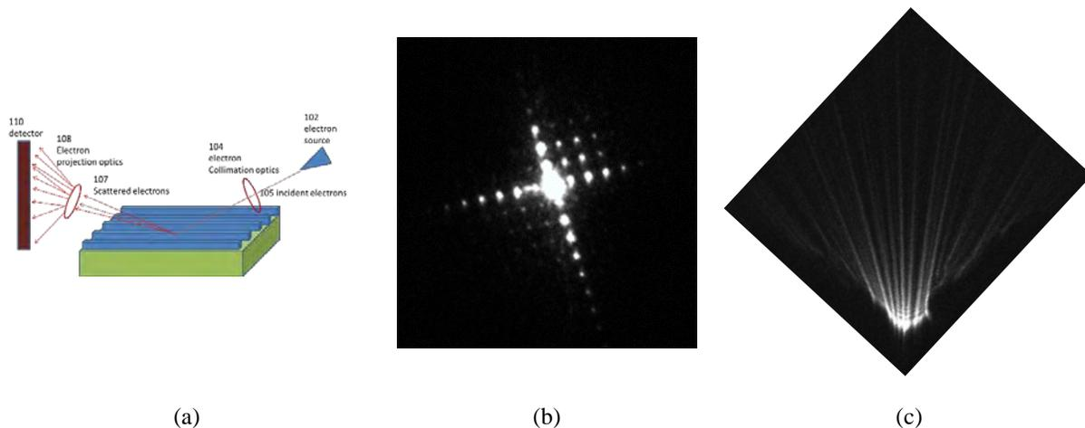
**FIGURE 1.** (a) Experimental setup for envisioned RSAES apparatus. (b) RSAES pattern from carbon film grating. (c) RSAES pattern from nanoscale Cu line grating.
