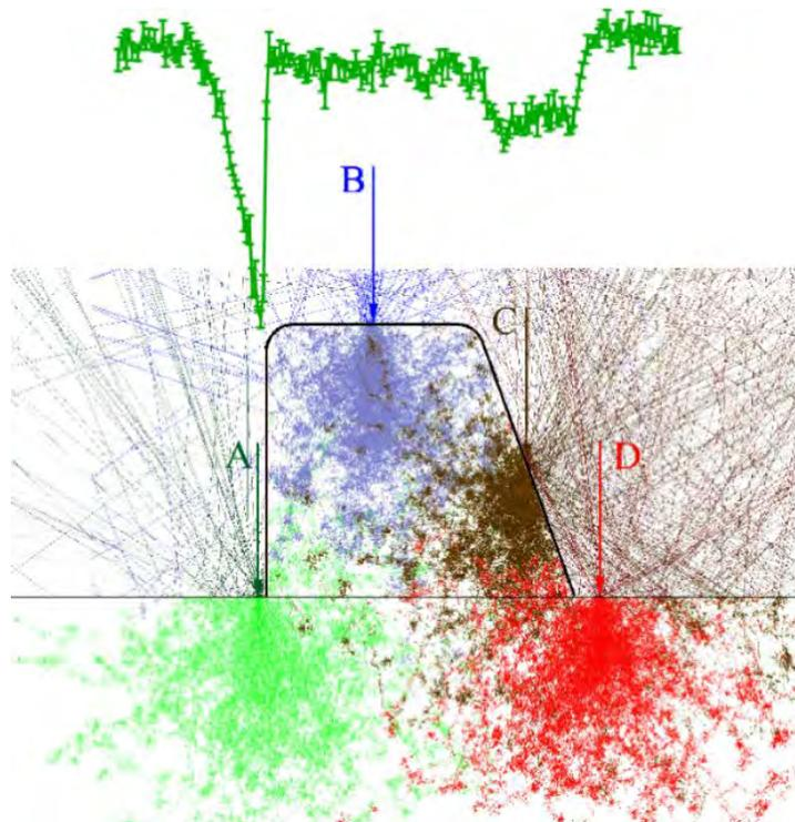
**FIGURE 1.** Model relationship of LLE signal to sample geometry. The upper (green) curve shows the modeled low-loss signal intensity from the line with near-vertical (left) and sloped wall (right) cross section shown in the lower portion. Electron trajectories at 4 landing positions, labeled A-D are superimposed on the sample geometry.
