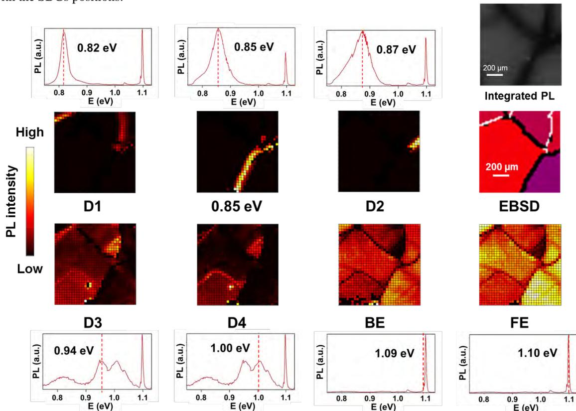
**FIGURE 4.**  $\mu\text{PL}$  intensity maps near sub-grain boundaries in “monolike” silicon showing the distribution of the well-known D-lines, the new line at 0.85 eV, the BE emission and the FE emission, on the same sample area at liquid helium temperature. Integrated PL map at room temperature and EBSD map are given on the same sample area. EBSD: white lines for low angle ( $<2 \text{ deg}$ ) disorientation, black lines for high angle ( $>2 \text{ deg}$ ) disorientation.
