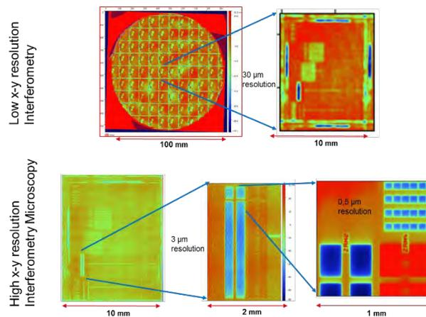
**FIGURE 2.** a) Low resolution Fizeau interferometer 100 mm scale data; b) Die level data extraction cm scale data c) high resolution PSI microscope Die level cm scale data d) in-die level μm scale data
