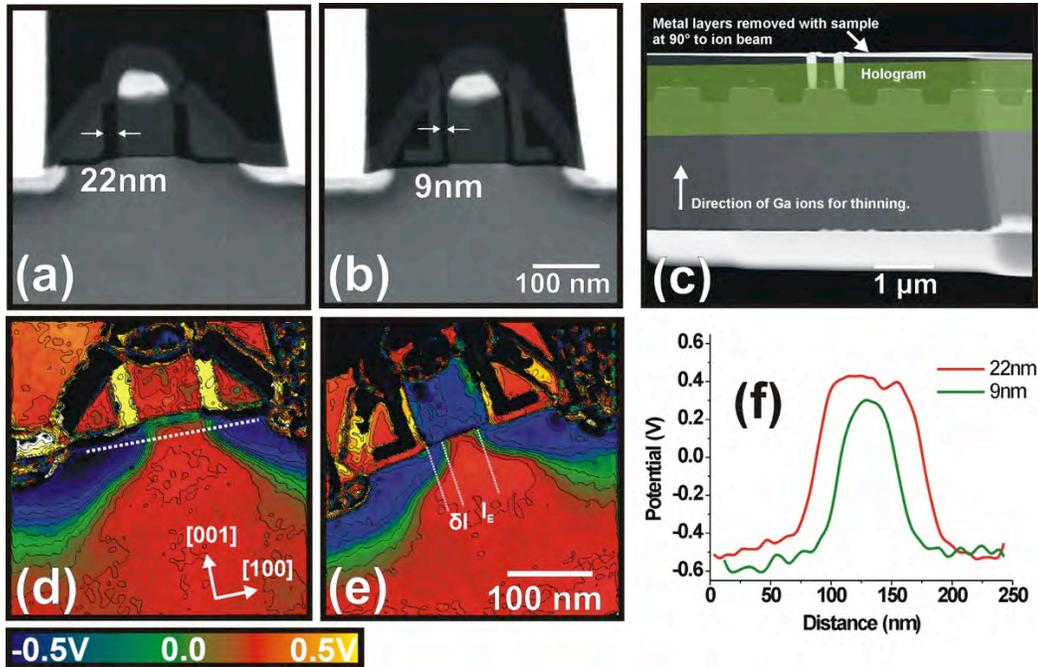
**FIGURE 1.** (a) and (b) show two p-MOS devices with different width spacers. (c) Electrically tested specimens have been prepared by back-side FIB milling. (d) and (e) show potential maps that have been acquired by off-axis electron holography. (f) Quantitative measurements of the electrostatic potential across the gate are shown.
