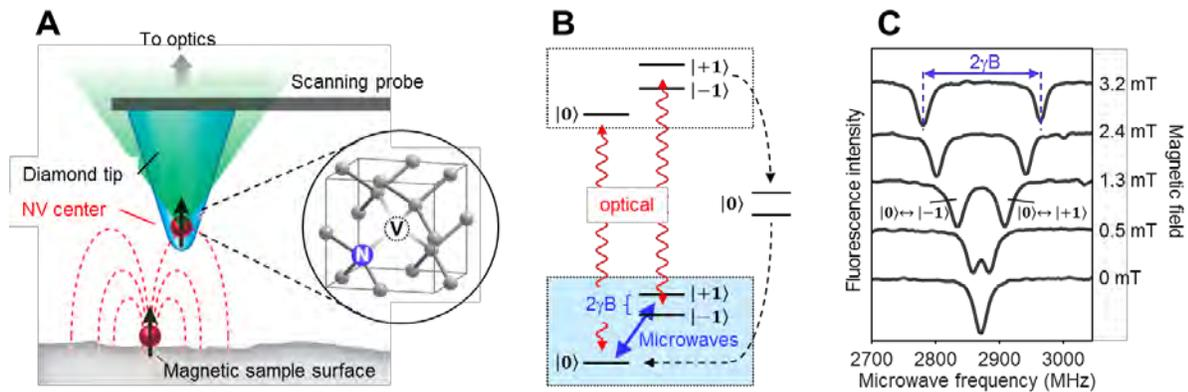
**FIGURE 1.** Basic principle of diamond-based magnetic sensing. (A) Scanning probe with an NV center at its apex. (B) Electronic and magnetic level structure of the NV center. A microwave transition (blue) is exploited for sensing. (C) Typical fluorescence response of an NV center when subjected to microwaves. The frequency of resonance peaks directly give the value of the local magnetic field.
