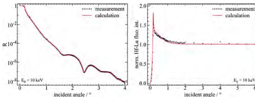
**FIGURE 1.** Comparison of conventionally modeled XRR of sample S4 800 °C (left side,  $\text{Al}_2\text{O}_3 / \text{HfO}_2 / \text{Al}_2\text{O}_3$  layer sequence) and the resulting GIXRF signal (right side) for Hf in comparison to the experimental data.
