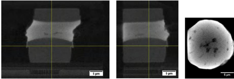
**FIGURE 2.** Three virtual 2D images (two perpendicular cross-section views and one planar view) through a solder connection (micro-bump of a HBM stack), based on a 3D data set from nano X-ray tomography. Imaging of a small extracted sample.
