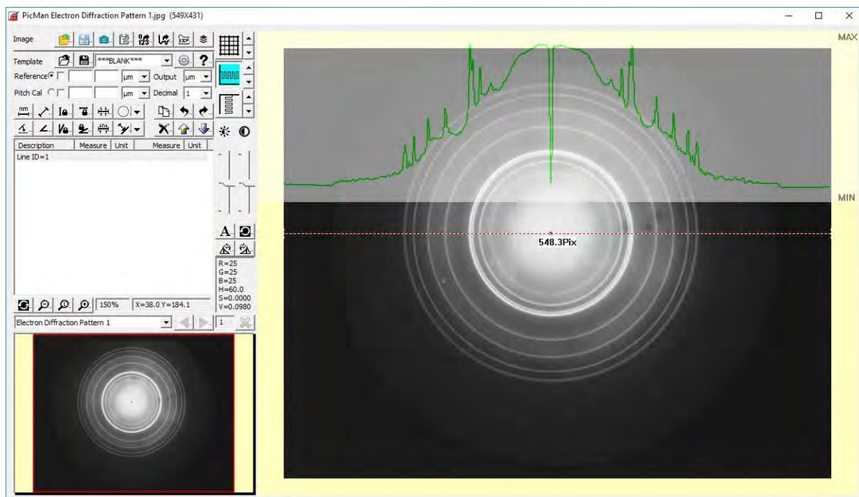
FIGURE 6. Electron diffraction image of microcrystalline specimen. [6]
