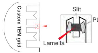
**FIGURE 4.** In-house fabricated customized TEM sample holder. A standard Cu-grid TEM holder is modified by FIB to create a small slit ( $\approx 2\text{-}3\ \mu\text{m}$ ) in the center of the middle pin, where the lamella will be placed and anchored by Pt deposited on the edges of the lamella.
