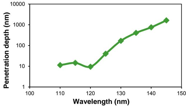
**FIGURE 2.** Penetration depth of silicon dioxide vs. wavelength. Note logarithmic vertical scale.
