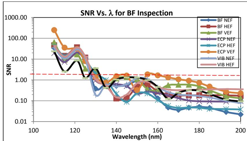
**FIGURE 4.** Simulation result of SNR for oxide over tungsten. A threshold of SNR = 2 is shown as a red dotted line. Note logarithmic vertical scale.
