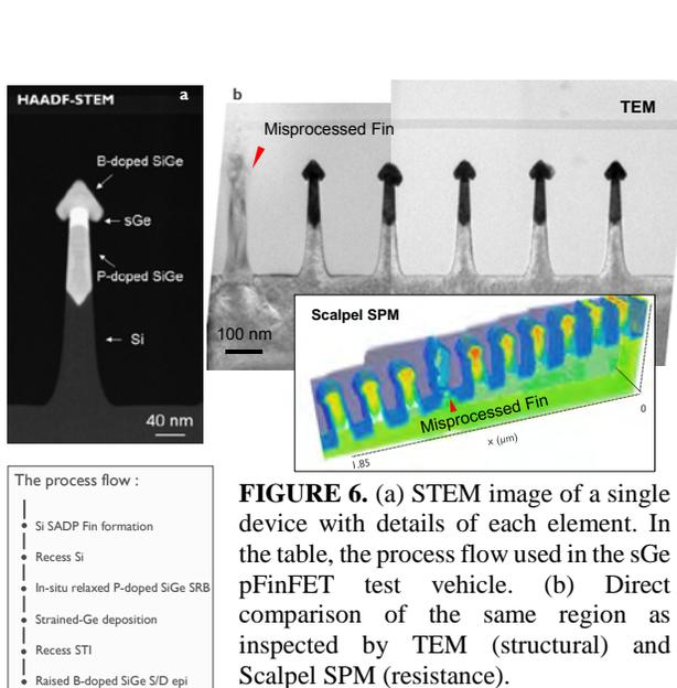
**FIGURE 6.** (a) STEM image of a single device with details of each element. In the table, the process flow used in the sGe pFinFET test vehicle. (b) Direct comparison of the same region as inspected by TEM (structural) and Scalpel SPM (resistance).
