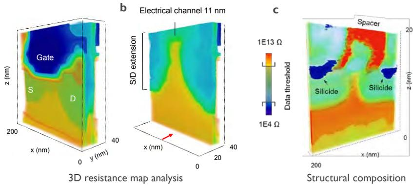
**FIGURE 3.** 3D-reconstructed volume of a single device visible at different stages along the y axis. (a) Out of the channel where the gate contact is visible and (b) under the gate where the spatial distribution of the S/D implants and the channel region are clearly visible. In addition, the other parts of the device are potentially accessible, for example in (c), filtering respectively the highest and lowest conductive features, the contact silicide and the spacer can be emphasized.
