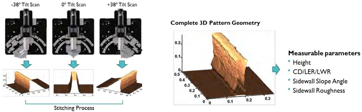
FIGURE 2. Schematic diagram of 3D AFM measurement method
