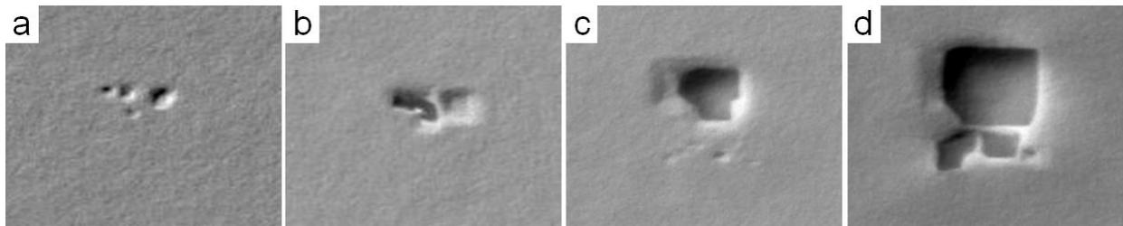
**FIGURE 2.** SEM images of the same defect at a: T1, b: T2, c: T3, d: T4.
