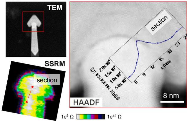
**FIGURE 9.** The pre-epi clean treatment applied before the growth of the doped-SiGe S/D, introduces a thin interfacial layer. Visible in both the TEM and the SSRM analysis, likely due to the residual strain or roughness between the sGe and SiGe. The conduction properties of this thin interface are visible in the SSRM profile where the interface shows a reduced conductivity. Clearly this interfacial layer increases the extension resistance of this transistor.
