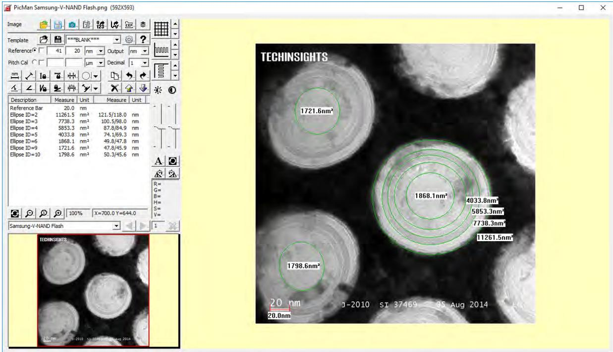
FIGURE 4. Plan view TEM image of 3D V-NAND device for area measurements. [4]
