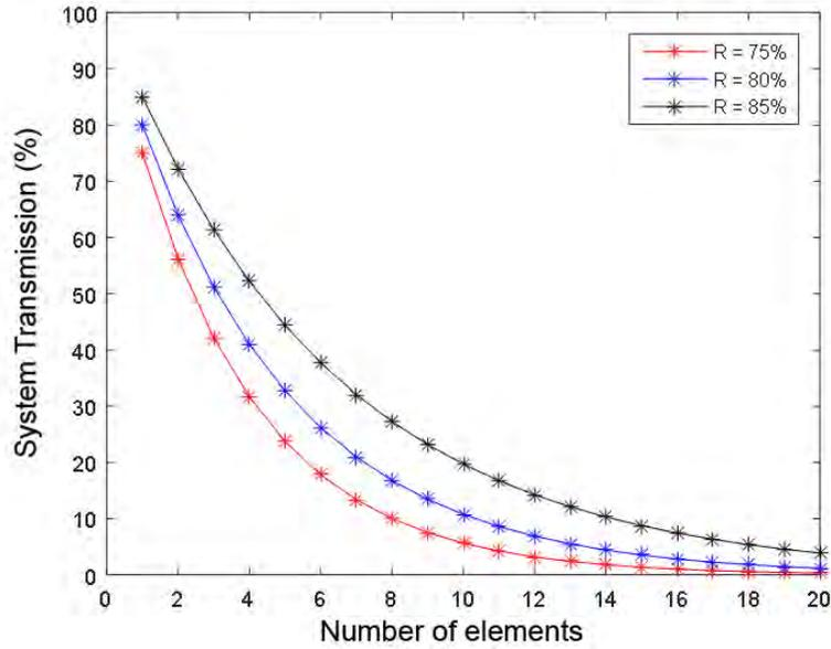
**FIGURE 9.** Total system transmission as a function of mirror reflectance and the number of mirrors employed in the system.
