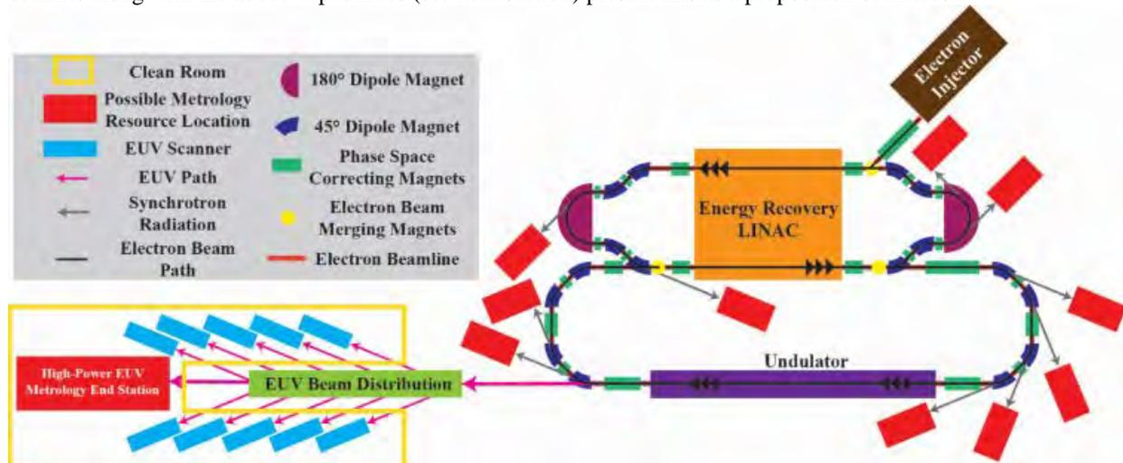
Figure 1. A conceptual schematic of an onsite ERL FEL design at GLOBALFOUNDRIES.
