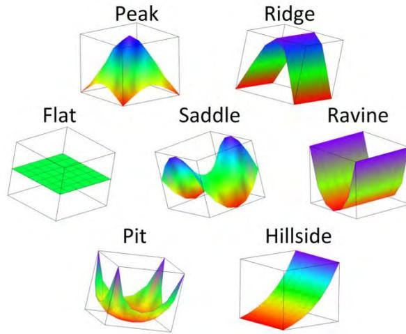
**FIGURE 2.** Surface patch labels. Pixels of 7x7 are classified according to characteristics.
