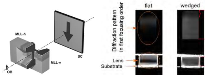
**FIGURE 6.** Crossed MLL after FIB preparation and assembly acting as a lens to image the object (OB) to the screen (SC) (left) [5] and diffraction patterns of flat and wedged multilayers (right).
