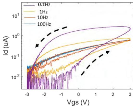
**FIGURE 2.** Experimental  $I_d$ - $V_g$  characteristics of polar polymer-based FeFET. 15 nm CP1 layer is incorporated as gate dielectric with 15 nm thick poly-Si layer used as the channel. The direction of observed hysteresis loop is schematically shown by arrows.
