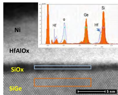
**Figure 4: STEM-EDS characterization of Al<sub>2</sub>O<sub>3</sub>-HfO<sub>2</sub> alloy/ Si<sub>0.7</sub>Ge<sub>0.3</sub>(001)/Si(001).** Blue box shows a region of interlayer for EDS revealing a Ge-free SiO<sub>x</sub> interlayer. The orange box is a control region in the SiGe. The EDS spectra of the interlayer is in blue while the spectra on the SiGe control region is in orange. Note the absence of Ge in the interlayer.
