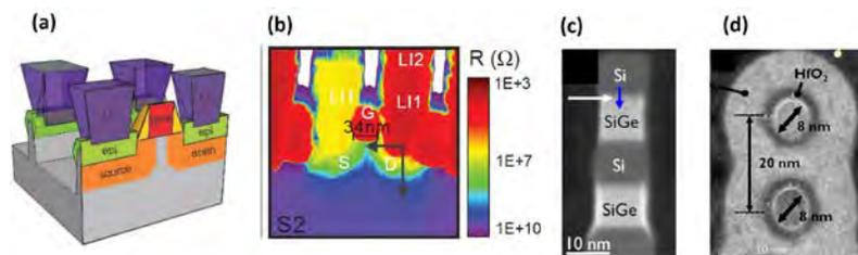
**FIGURE 1.** (a) Cross-section of scaled FinFET showing gate, electrodes, and junctions. (b) 2D SSRM resistance maps for FinFET sample. (c) Si-SiGe Super lattice fin necessary to produce the Gate-All-Around Nanowires as should in (d). Sources: 1(a),(b) from Ref. 1, 1(c) and (d) from Ref. 2.
