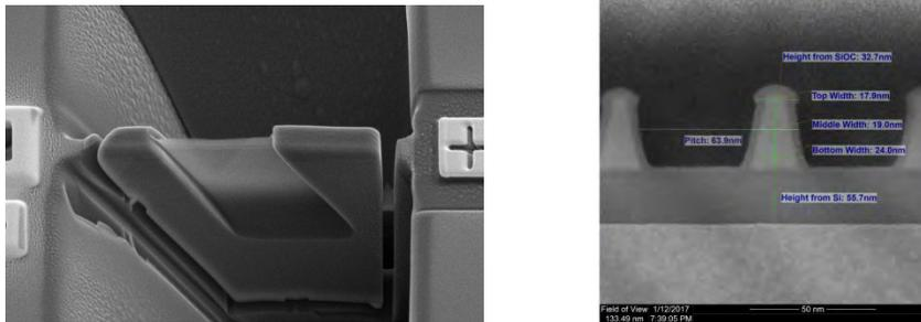
**FIGURE 2.** (a) Lamella after automated FIB sample prep on the wafer, (b) Automated Metrology on TEM images.
