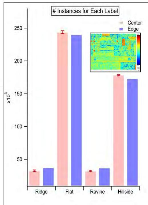
**FIGURE 4.** Distribution of surface patch labels for a measured region of interest (inset) in a die. Center and edge are compared which show a difference.
