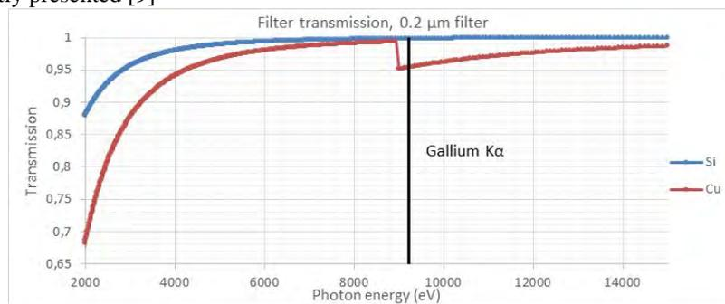
**FIGURE 3.** X-ray transmission through a 0.2  $\mu\text{m}$  filter of silicon and copper. The black line indicates the  $K\alpha$  of gallium [8].
