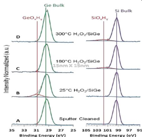
**FIGURE 1:** In-situ XPS in UHV of HOOH(g)/Si<sub>0.5</sub>Ge<sub>0.5</sub>(001). Dosing with HOOH(g) induces only a GeO<sub>x</sub> component. Annealing removes the GeO<sub>x</sub> and only a SiO<sub>x</sub> component is formed.[2]
