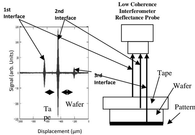
**FIGURE 1.** Measured asymmetric interferogram exhibits strong peaks corresponding to boundaries in the measured structure.
