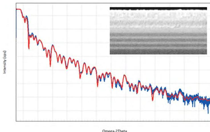
**FIGURE 2.** XRR from SiGe/Si nanosheet on a bulk Si substrate. Analysis of the measured data provides information on the individual layer thickness, density, and interfacial width (roughness). The measured intensity profile (blue) is overlapped with the best fit simulation (red). Comparison with a destructive SEM cross-section (inset) shows good thickness correlation.
