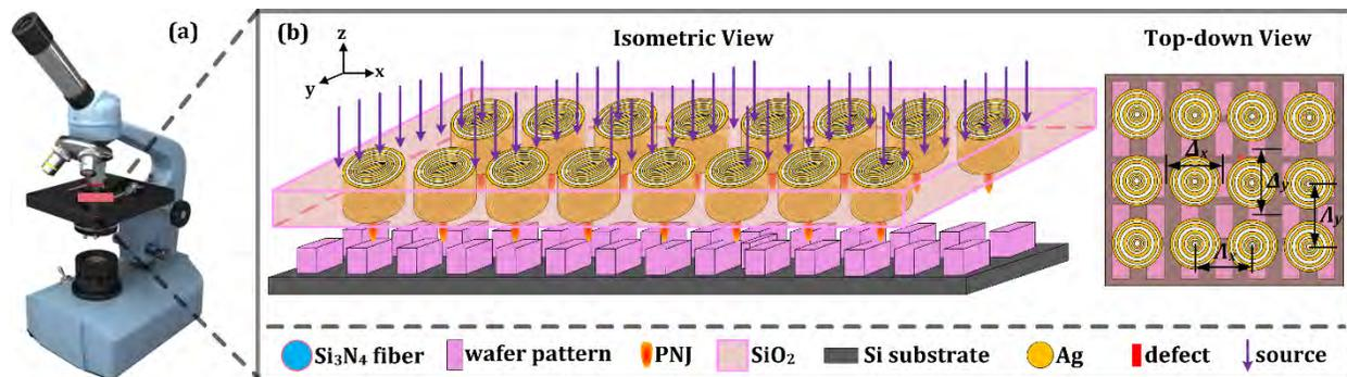
**FIGURE 1.** (a) Illustrated diagram showing a coherent optical microscope and (b) the mechanism of the metalens array-assisted defect detection system.
