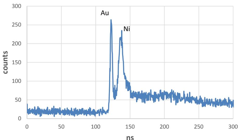
**FIGURE 2.** Time of flight spectrum of 0.7 nm Au on 2.7 nm Ni on Al<sub>2</sub>O<sub>3</sub> taken with a 10 μm beam spot size and uncorrected for finite detector size and kinematic effects.
