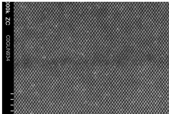
**FIGURE 2:** TEM micrograph of (bottom to top) Si, monolayer, overgrown Si; the crystallinity is clear, but where exactly is the interface?
