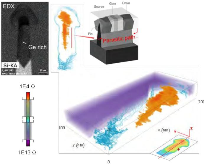
**FIGURE 11.** The mid-range and high resistive features are suppressed in the 3D tomogram (resistance map) according to the color-scale, to highlight the extension and 3D evolution of the defective area inside the SRB (3D cut as in the bottom inset). The top-right schematic describes a potential parasitic path introduced by such kind of defective SRB. A similar effect has been often ascribed to the threading dislocations density in the P-doped SiGe.
