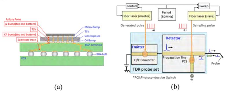
**FIGURE 2.** (a) Advanced semiconductor package structure and typical fault locations. (b) Schematic diagram of the developed TDR transceiver and TDR signal generation/sampling scheme.
