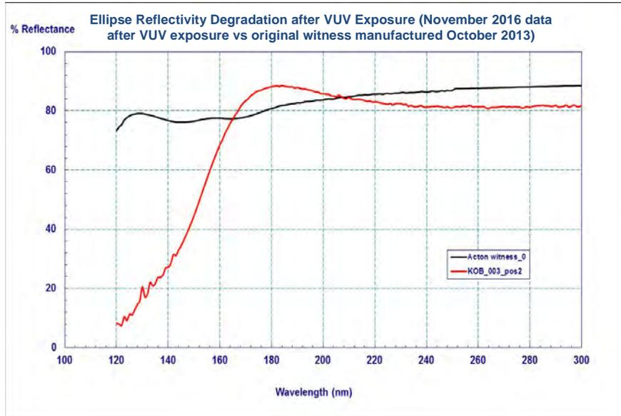
**FIGURE 6.** VUV degradation of the reflectance of protected aluminum. Unexposed sample (black); exposed sample (red).
