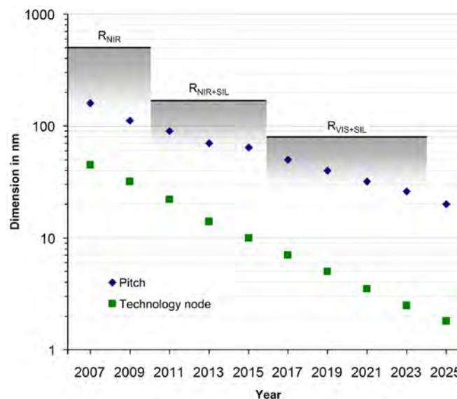
**FIGURE 1.** Technology generations with their FET pitch sizes according to ITRS roadmap [3]. Grey areas indicate fault isolating capability in real world IC debug with NIR and NIR+SIL based on [1] and adapted for VIS+SIL (after [6]).
