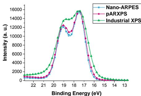
FIGURE 2. Comparison of Hf4f XPS spectra obtained by Nano-ARPES, pARXPS and industrial XPS.
