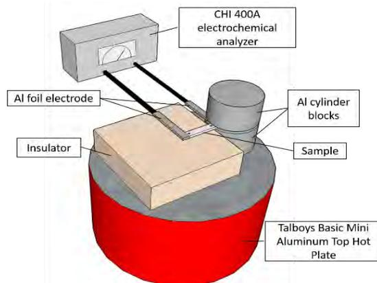
**FIGURE 1.** Schematic of the Self-built Seebeck Coefficient Measurement Apparatus.
