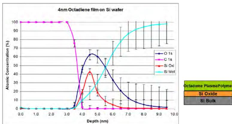
**FIGURE 1.** Maximum entropy modeling results from ARXPS data from an octadiene plasma polymer film deposited on the native oxide of a silicon wafer.
