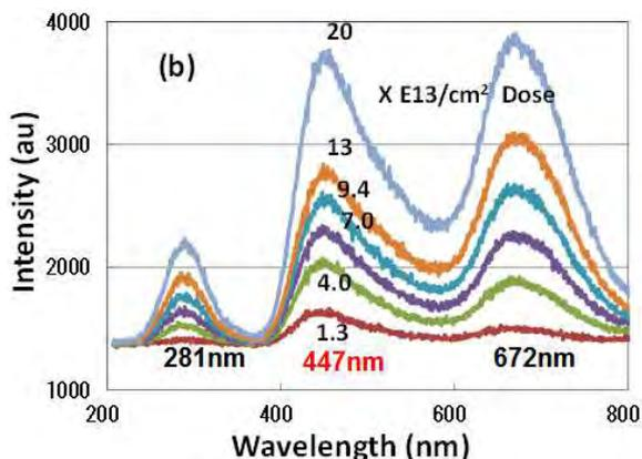
FIGURE 1. Helium ion beam induced luminescence spectra from SiO<sub>2</sub> at different ion doses of 1.3-20 E13/cm<sup>2</sup> at 30kV.
