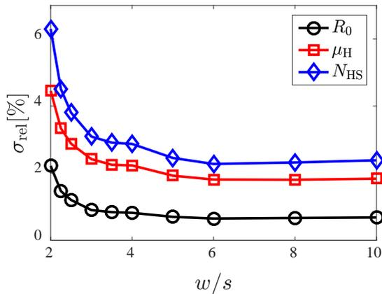
**FIGURE 2.** Relative standard deviation for  $R_0$ ,  $\mu_H$  and  $N_{HS}$  vs. width,  $w$ , of the test pad in question. The probe is placed at  $y_0 = 0.4s$  and the length,  $L$ , of the test pad is  $7s$ . The relative standard deviation is seen to increase below  $w=3.5s$ .
