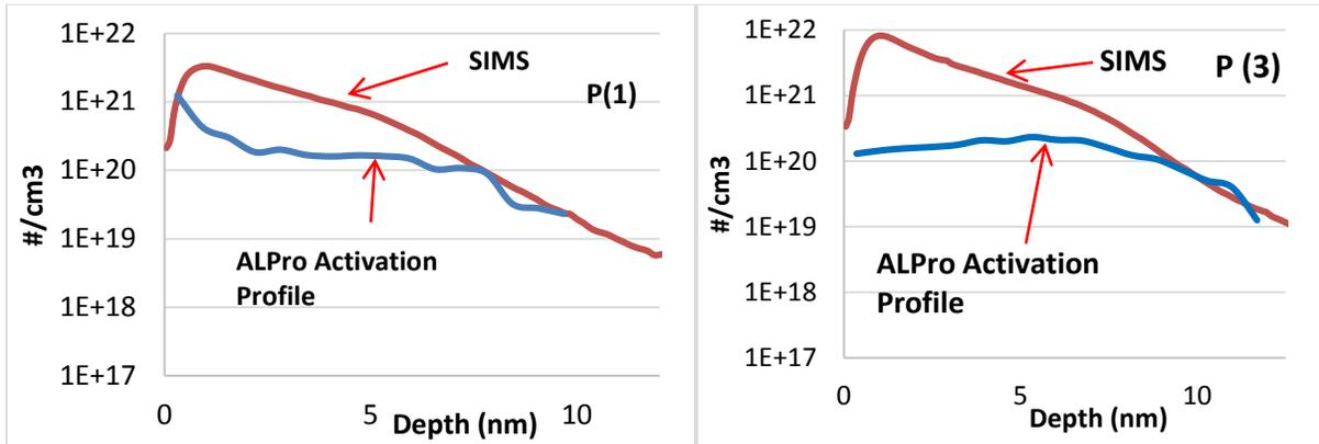
**FIGURE 1.** Samples: P1 =  $1 \times 10^{15}/\text{cm}^2$  Phos-doped Silicon and P1 =  $3 \times 10^{15}/\text{cm}^2$  Phos-doped Silicon. The post-anneal SIMS ‘as-is’ dopant profile, and ALPro Activation profile.
