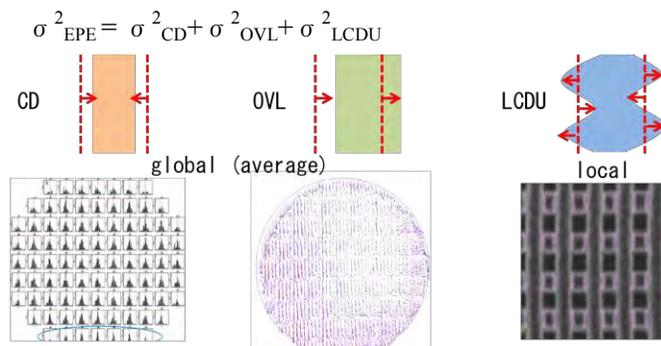
FIGURE 1. Edge placement error measurement requires global and local CD measurement
