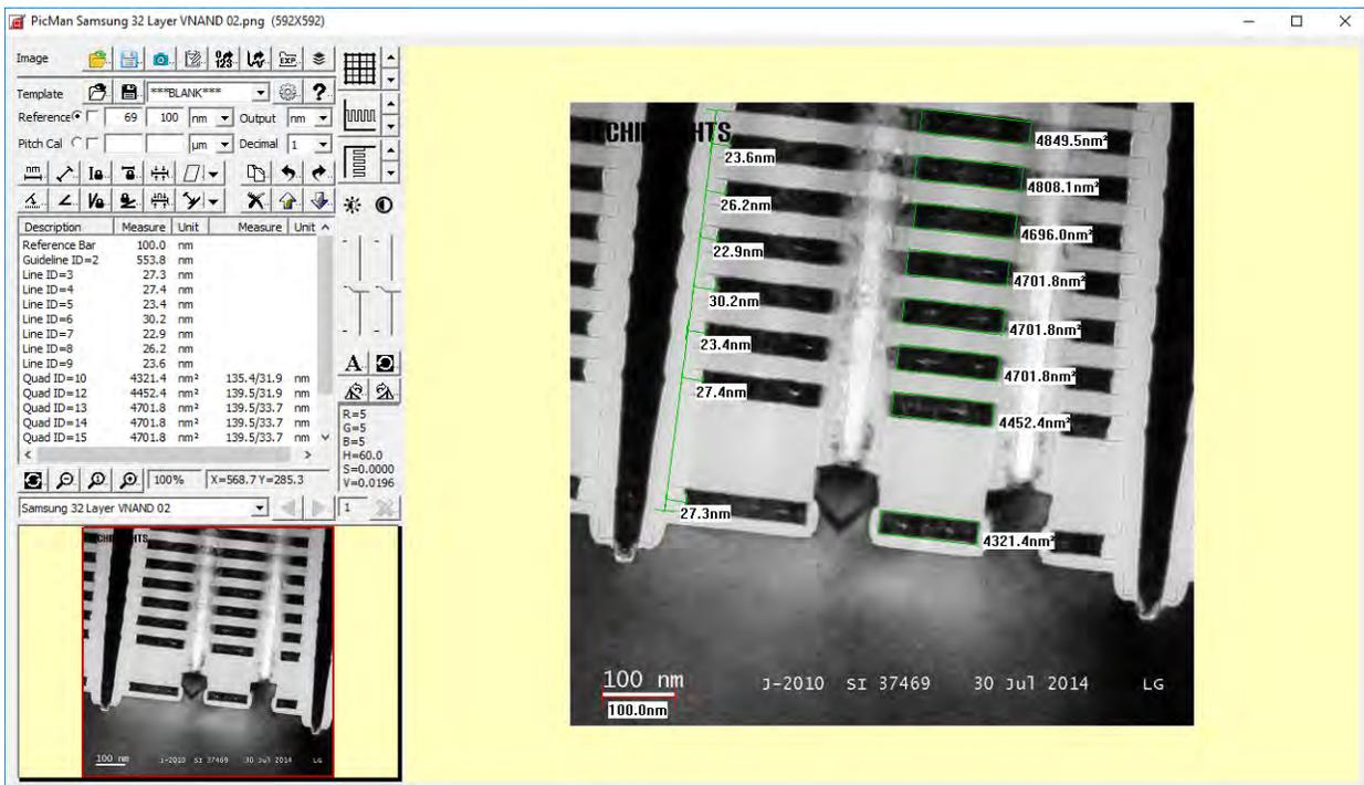
FIGURE 3. Cross section of a 3D V-NAND device (high magnification image). [3]
