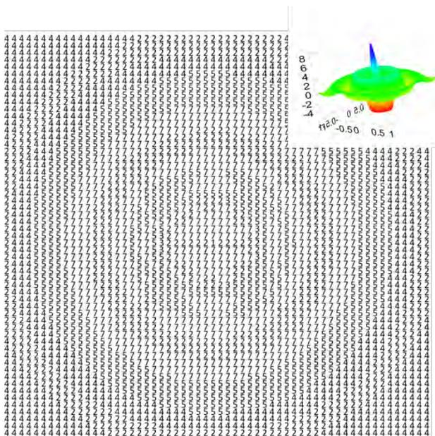
**FIGURE 3.** Surface patch labels for a test structure (inset) whose characteristics are known. Note the peak (1) at the center and ridges (2) and ravines (5) in concentric regions.
