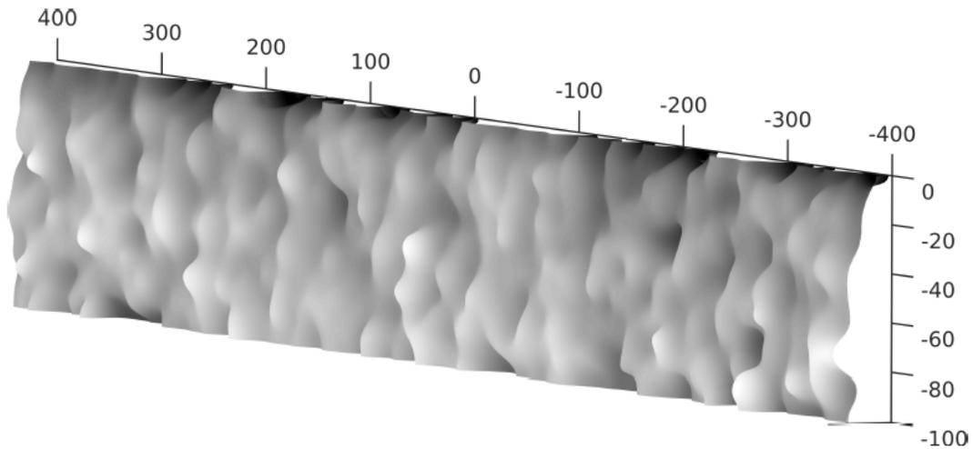
**FIGURE 3.** A three dimensional view of the boundary between exposed and unexposed resist. The surface is obtained from a simulated exposure of a 100 nm thick layer of CAR on an infinitely thick silicon substrate, assuming a Poisson distributed exposure dose of 40  $\mu\text{C}/\text{cm}^2$ .
