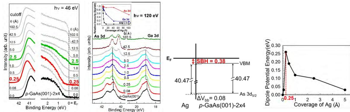
**FIGURE 3.** (Leftmost) Valence-band spectra in the vicinity of the Fermi level ( $E_F$ ) and low-energy cutoff recorded with a photon energy of 46 eV for Ag on a  $p$ -GaAs(001)-2x4 surface.
