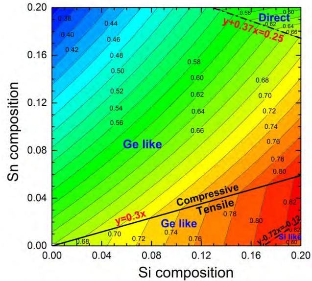
**FIGURE 1.** Compositional dependence of the lowest band gap (either direct or indirect) of pseudomorphic  $\text{Ge}_{1-x-y}\text{Si}_x\text{Sn}_y$  on Ge.
