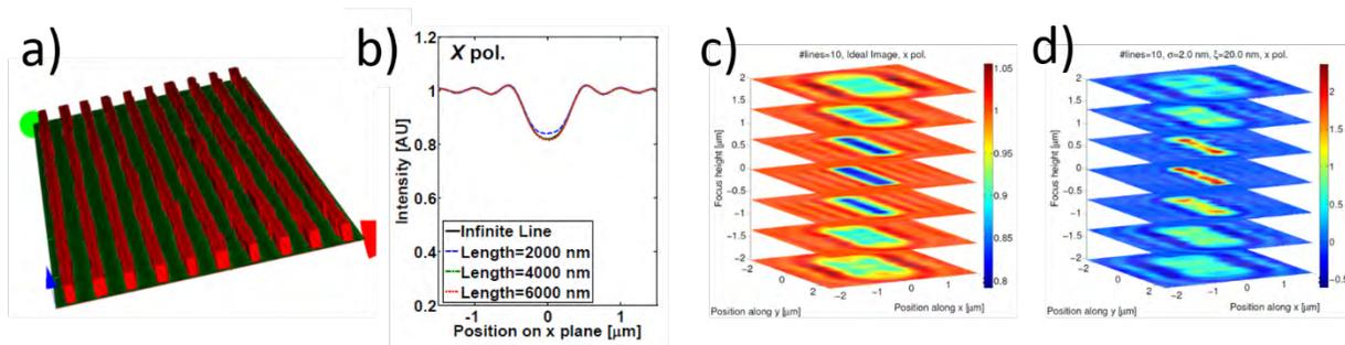
**FIGURE 3.** a) Single realization of a rough 10-line structure. b) Comparison between the profiles of the infinite and finite lines for three different line lengths  $l_y$  for a 10-line target at  $\lambda = 450$  nm. c) Images of the ideal, i.e. non-perturbed 10-line structure at several focus positions. d) Relative difference between the image of ideal and rough 10 line structures at several focus positions.
