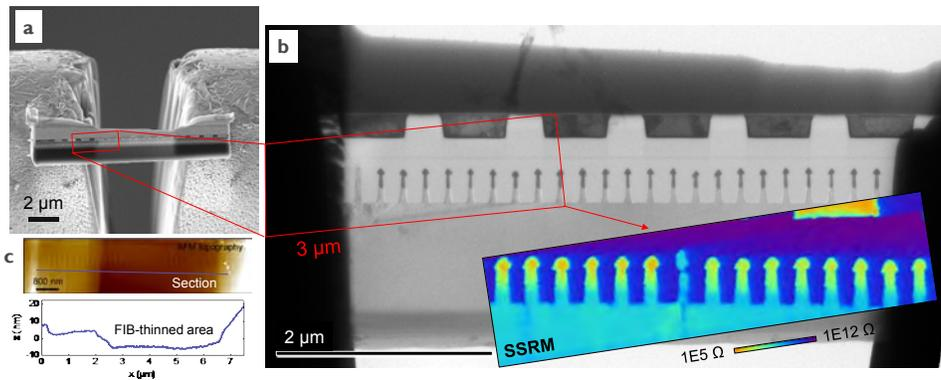
**FIGURE 5.** (a) SEM image of the lamella as mounted on the custom TEM grid. (b) SSRM and TEM can be alternatively used on the area of interest (red box). The SSRM image of a series of structures is combined with the high resolution TEM image. (c) AFM is used to image the surface of the sample. Note in the AFM profile the step associated to the FIB-thinned region in the middle part of the lamella.
