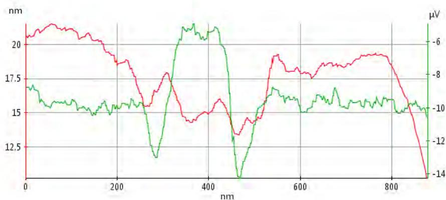
**FIGURE 2.** Line profiles of the AFM topography (red, left y-axis in nm) and the capacitance data (green, right y-axis in  $\mu\text{V}$ ) of the Device 4 area scanned in Figures 1 and 3.
