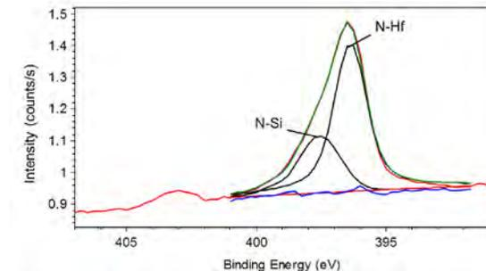
**FIGURE 4.** N1s XPS spectra obtained on the in-line XPS and the measurement program modeling.
