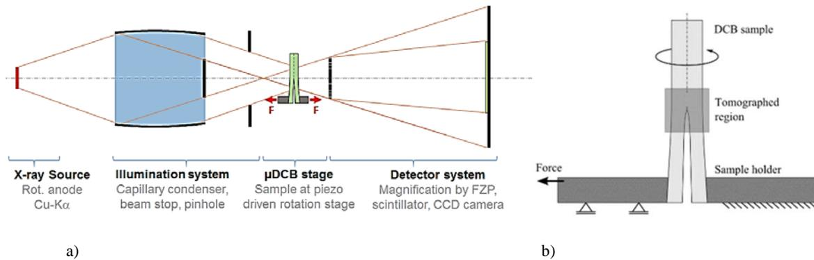
**FIGURE 2.** a) Scheme of microDCB test setup inside a nano-XCT tool, b) schematic drawing of microDCB test setup [1]
