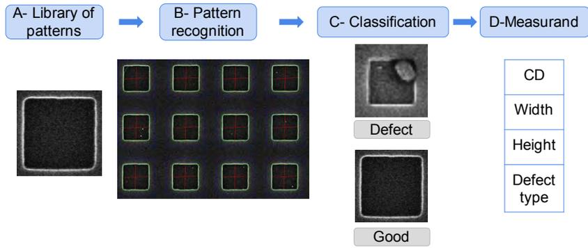
**FIGURE 5.** Machine learning sequence from library set-up on the left side to pattern recognition, classification and final measurements on the right side.
