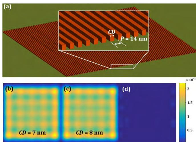
**FIGURE 2.** Simulations show the extremely low sensitivity of the far-field image to the CD of a line array. (a) Illustrated diagram showing the geometry of the patterned nanostructure. Simulated far-field signals for a (b) 7 nm and (c) 8 nm CD, respectively. (d) Difference signal obtained by subtracting Fig. 2(b) from Fig. 2(c).
