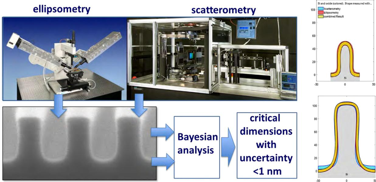
**FIGURE 1.** Left: scheme of a hybrid measurement approach: goniometric scatterometry and spectroscopic ellipsometry measurement data are combined in a Bayesian analysis to provide CD values with reduced measurement uncertainties; right: measurement results obtained with DUV (266 nm) reflectance measurements (blue), spectroscopic ellipsometry (red) and a hybrid analysis (yellow) of Si-gratings with nominal CD/pitch values of 25/50 nm (top) and 50/100 nm (bottom).
