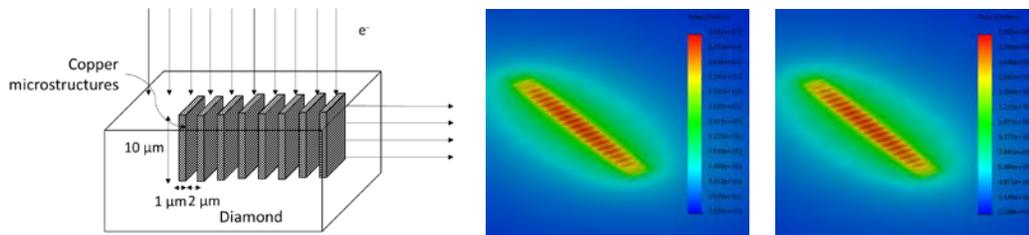
**FIGURE 5.** Scheme of the microstructured target of the Sigray Fine Array Anode Source Technology (FAAST™) source (left) as well as thermal modeling of the Sigray FAAST™ (middle) and of a conventional Cu X-ray target (right)
