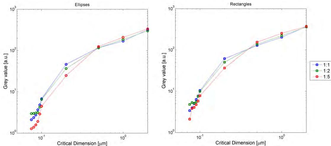
**FIGURE 4** The measured RN3.9 signal strength as a function of the CD of a gold ellipse (left) and rectangle (right) on a Si wafer for aspect ratio's (AR) 1:1, 1:2 and 1:5. The AR has a significant impact on the DF scatter signal strength, leading to an under-estimation of the CD for defects <500 nm when using an “equivalent” sphere.
