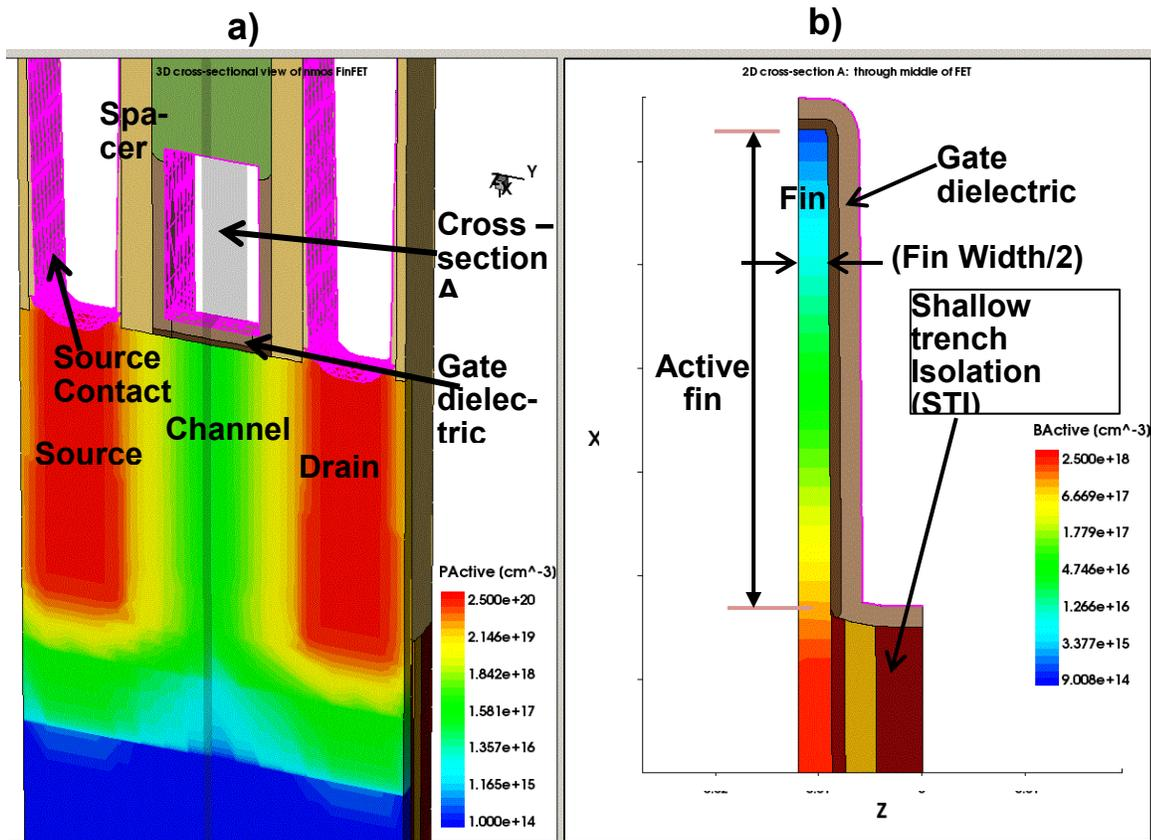
FIGURE 1. (a) 3D FinFET cross-section (b) 2D cross-section A from Figure 1a, showing a slice through the middle of the FET
