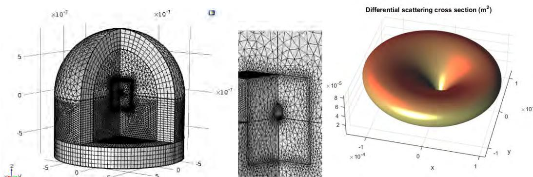
**FIGURE 2** Geometry (left and center panel) and scattering profile (right panel) for typical RN3.9 illumination conditions. The differential scattering cross section calculated with an analytical model for a 30nm-radius spherical Au particle on a Si substrate illuminated by p-polarized light coming in at a 60° angle.
