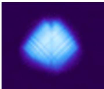
**FIGURE 1.** Image of the x-ray beam at a source to detector distance of 418 cm.
