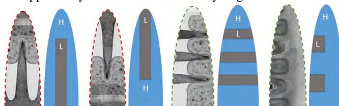
**FIGURE 1.** FinFET analysis options alongside the resulting simplified, evaporation field variation expected for four considered orientations with the fin as the ROI (blue=high field, gray=low field). From left to right: top-down, backside, parallel to the gate, and parallel to the fin.
