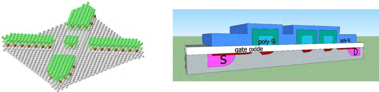
**FIGURE 1.** Two prototypical devices: Left: single-atom device with electron localized to P+ dopants (color: red, B/W: dark dots); dopants are surrounded by crystalline Si. Right: quantum dot device with two-dimensional electron gas (2DEG) (color: red, B/W: black) at interface between Si and oxide.
