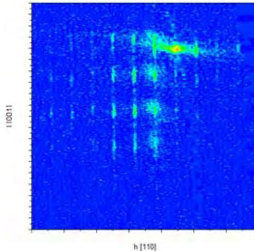
**FIGURE 3.** HRXRD reciprocal space map (RSM) in the vicinity of the 113<sub>g</sub>e Bragg reflection of fins etched into a nanosheet stack on Si(001) substrate.
