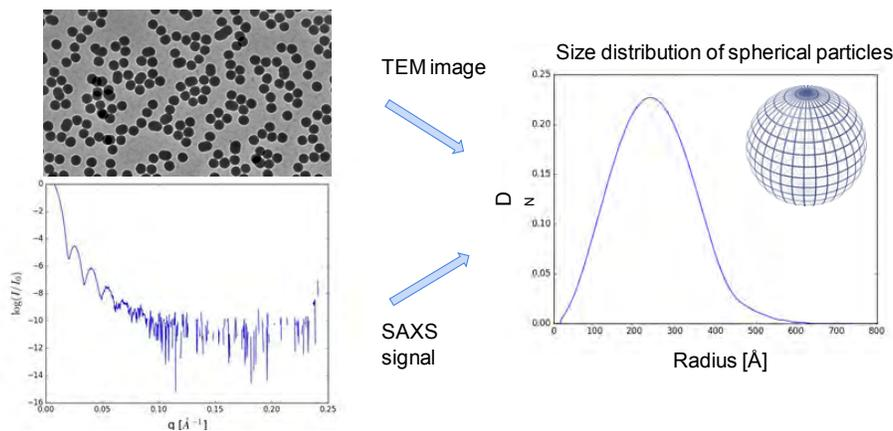
FIGURE 4. Data fusion of a direct (TEM) and an indirect (SAXS) measuring technique, giving rise to a new measurand, here the size distribution.
