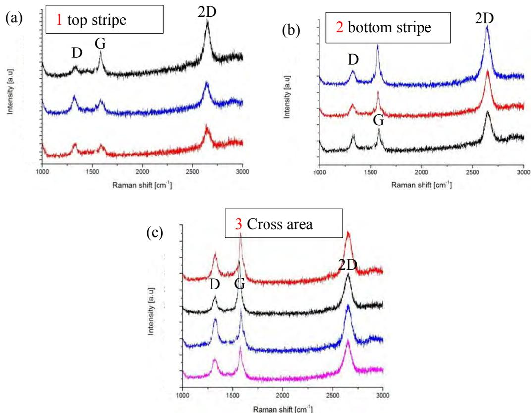
**FIGURE 2.** Raman shifts measured from (a) top graphene stripe (b) bottom graphene stripe, and (c) the two graphene stripes crossed or contact area.
