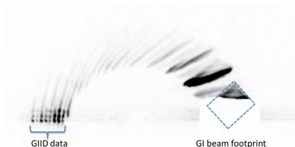
**FIGURE 2.** CCD detector image of data collected on a NIST Si Fin structure using the CLS to explore a new method for GI in-plane diffraction (GIID). The CLS beam was focused at the sample with a K-B multilayer (shown as a footprint of direct GI beam outlined in the box). The sample is rotated in-plane to reveal strong scattering resonances near grazing incidence. Note the sample itself is acting as an angular filter.
