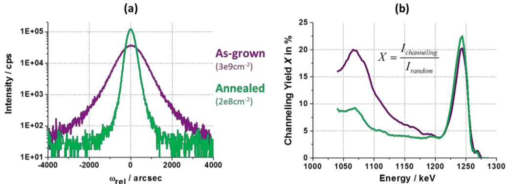
**FIGURE 1.** (a) Omega rocking curve obtained on blanket Ge layers of different threading dislocation densities (TDD). (b) RBS channeling yield measured on the same Ge layers.
