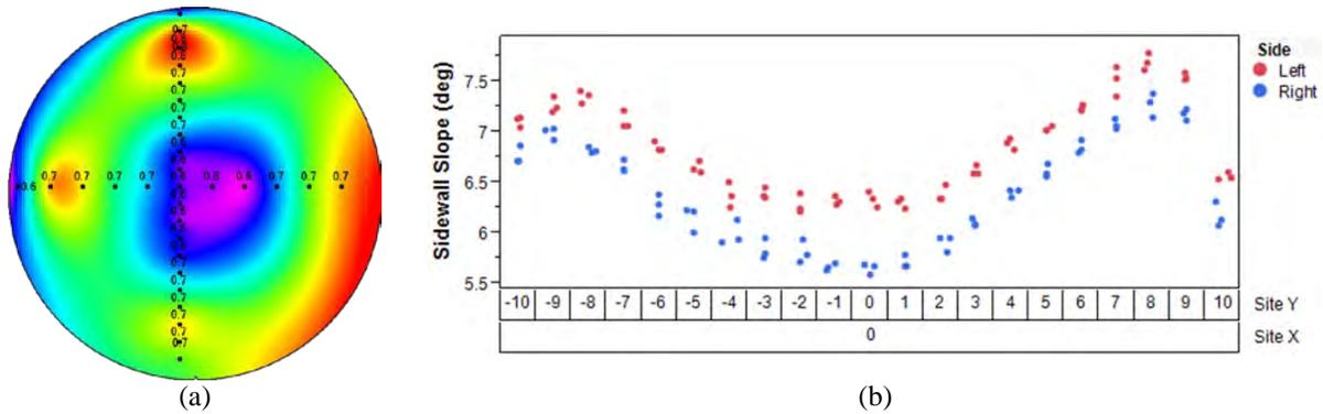
FIGURE 5. (a) Wafer map of sidewall slope and (b) their value change on Y axis of wafer
