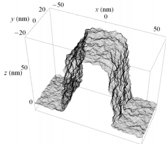
**FIGURE 1.** Line drawing of the roughest of our 3 virtual samples. The line is oriented to show the right edge. The left edge is obscured by absence of hidden line removal.
