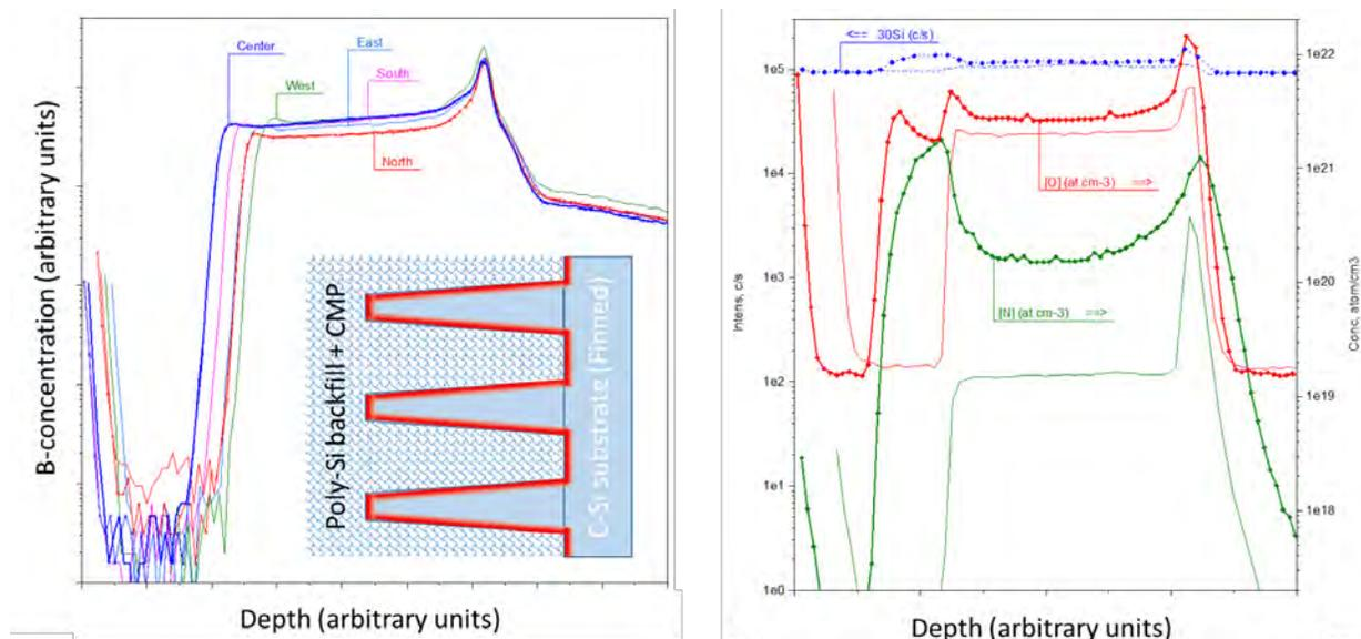
**FIGURE 1.** panel a (left): 1.5D SIMS B-profiles on Fin arrays from different wafer locations after Boron plasma doping and subsequent RTA, cleans / poly-Si backfill / CMP, and panel b (right): 1.5D SIMS N and O profiles on Fin array with (symbols) and without (no symbol) SiNx residual hardmask
