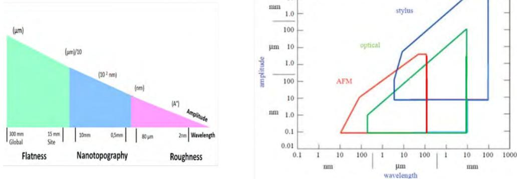
**FIGURE 1.** a) Nanotopography domain in spatial wavelength and amplitude; b) wavelength and amplitude of different surface topography instruments.
