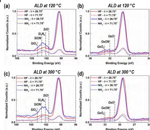
**FIGURE 2:** Angle Resolved XPS of HF(aq) vs NH<sub>3</sub> plasma passivated SiGe(001) with 8 cycles Al<sub>2</sub>O<sub>3</sub> ALD at 120 °C vs 300 °C. Note: At 300 °C, there is no GeON component [5].
