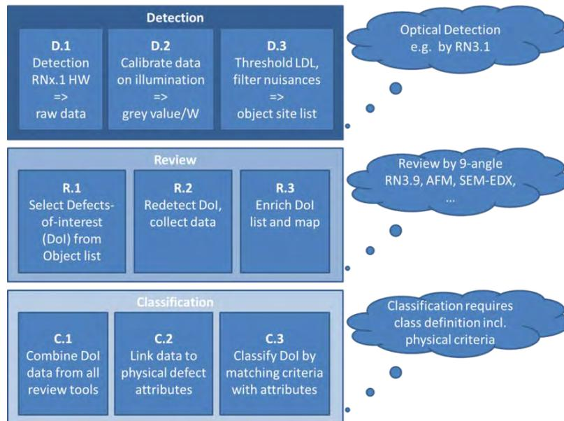
**FIGURE 1** Process flow for the detection, review and classification of defects.
