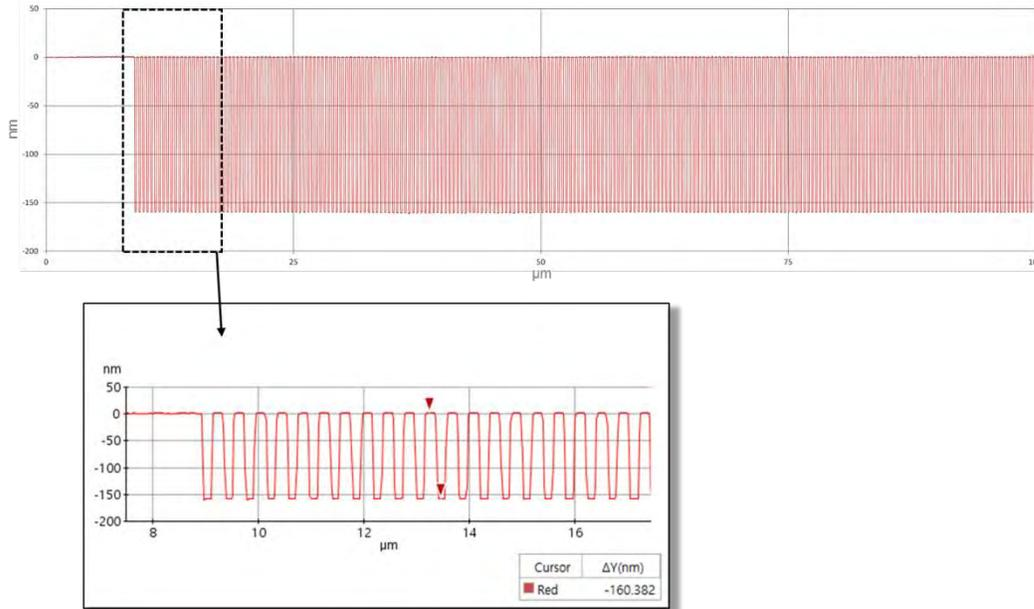
**FIGURE 1.** The small-scale profiling using XY scanner. The range is 100  $\mu\text{m}$  and the step height is 160 nm. The inset shows a magnified section of the same profile.
