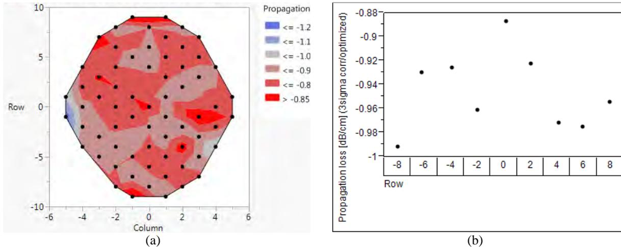
**FIGURE 7.** (a) Wafer map of propagation loss, measured at the wavelength of 1550 nm and (b) their value change on Y axis of wafer
