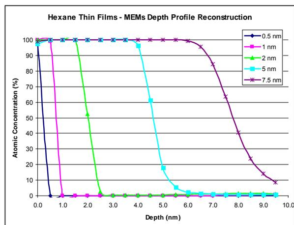
**FIGURE 2.** ARXPS/MEMs results from varying thicknesses of hexane plasma polymer films on silicon wafers, showing the thickness measurement capability inherent in the technique.
