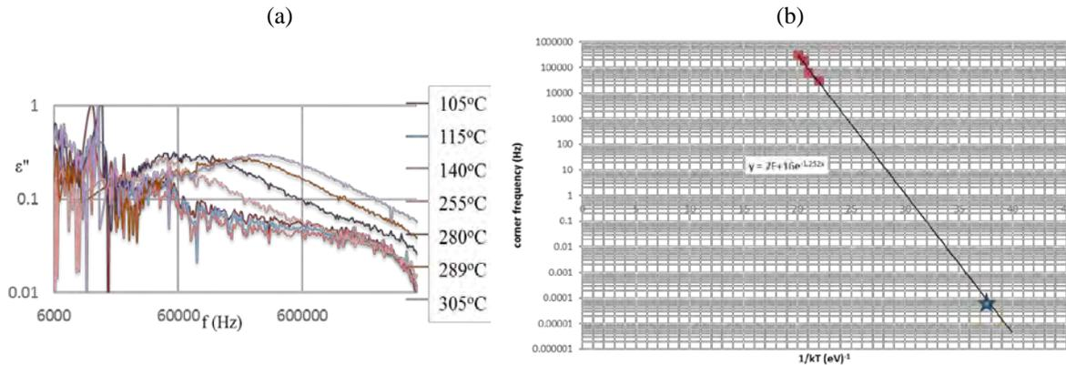
**FIGURE 1.** (a) Dependence of the measured imaginary part of the dielectric constant vs. frequency at different temperatures. MIM structure with 11nm thick CP1 was used. (b) Dependence of the peak frequency of the  $\epsilon''(f)$  spectra vs.  $1/kT$  and the theoretical fitting to the experimental data (solid line). Expected value of peak frequency at room temperature is shown by the star symbol.
