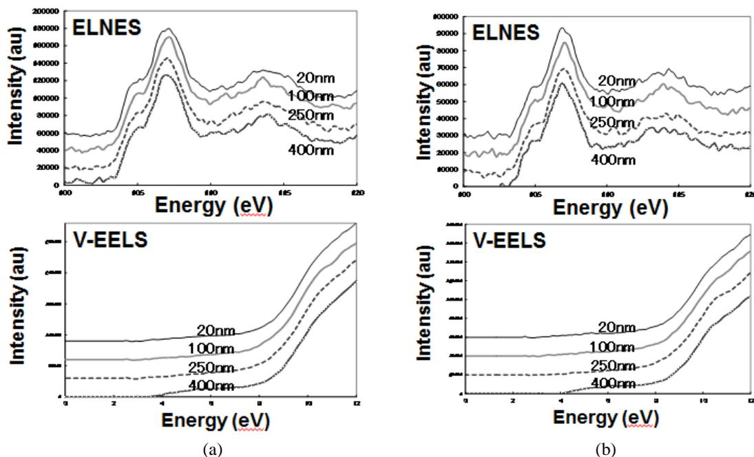
FIGURE 2. TEM ELNES and V-EELS spectra at distances of 20, 100, 250, and 400 nm from the SiO<sub>2</sub> surface without helium ions beam irradiation (a) and with 2E14/cm<sup>2</sup> helium ions beam irradiation (b).
