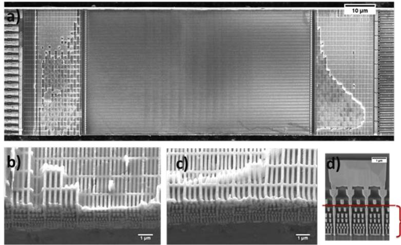
**FIGURE 4.** SEM images: a) overview of the fracture surface with two fractured crack stop structures, and at higher magnification b) and c); d) comparison of the number of the damaged layers with non-damaged structure.
