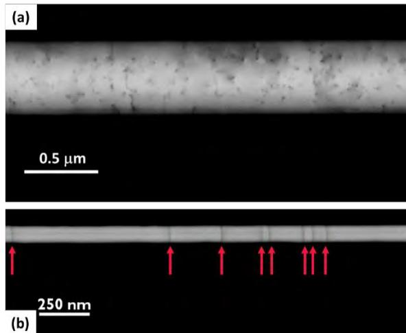
**FIGURE 4.** (a) Threading dislocations and (b) stacking faults in SiGe fins visualized by ECCI
