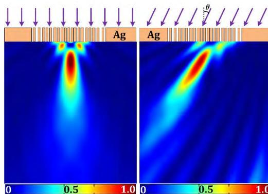
**FIGURE 2.** Focusing characteristics of the designed metalens. The intensity maps are obtained by setting the incident angles as (a)  $0^\circ$  and (b)  $30^\circ$ , respectively. Metalens height: 215 nm. Slit widths: 10-30 nm. Material in slits: air. All the sub-figures have been normalized by the maximal intensity.
