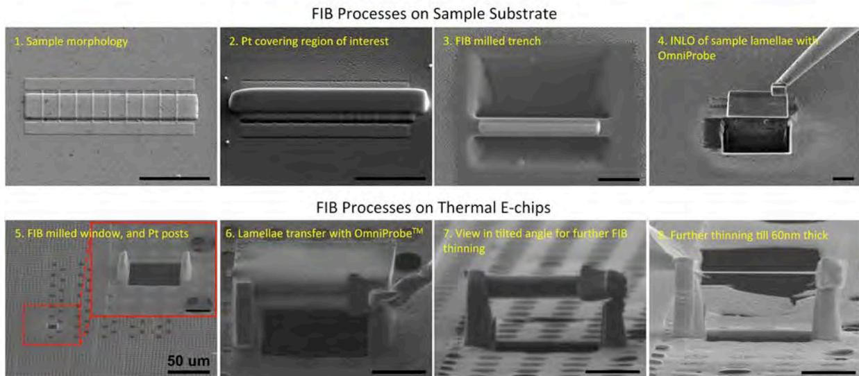
**FIGURE 1.** SEM images show the fabrication sequences to transfer the FIB cut lamellae from the home substrate onto the TEM membrane window of a TEM compatible thermal chip. All the scale bars are  $5\mu\text{m}$ , except the one labeled separately in step 5.
