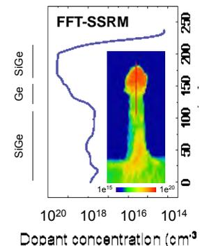
**FIGURE 8.** Due to the parasitic terms introduced by the small geometries (very high series resistance), FFT-SSRM is used for the direct quantification of the carriers in the SiGe-based raised S/D regions.
