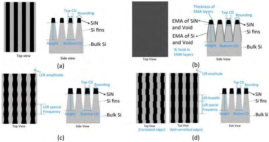
**FIGURE 1.** Different methods of including Line Edge Roughness are shown. 1.a shows idea lines with no LER. 1.b shows the use of and effective medium layer to model LER. 1.c shows a non-random sinusoidal line edge. This method proved to be the most successful 1.d shows a line segment off-set approach. [2]
