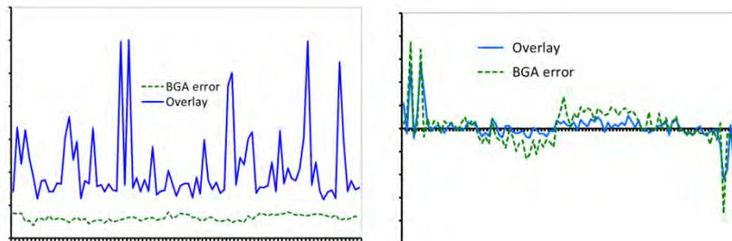
**FIGURE 4.** measured results of BGA-induced error (green curve) and measured overlay (blue curve) on product wafers. The left graph shows a case where grating asymmetry is quite stable (jumps in overlay are not related to BGA) and the right graph shows how a varying bottom grating asymmetry impacts the measured overlay.
