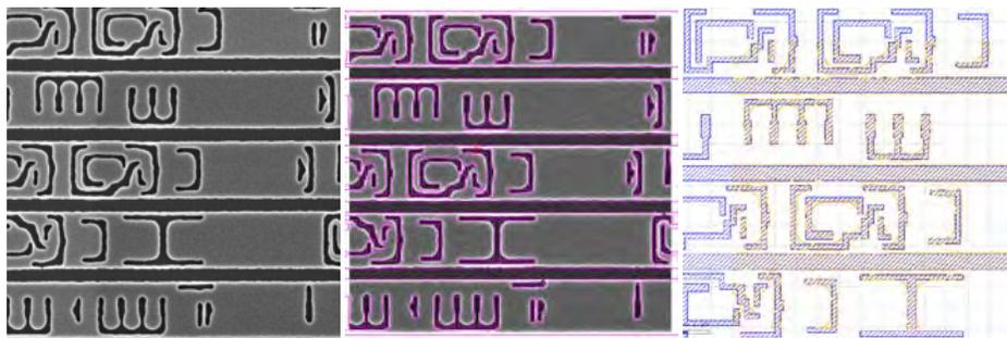
FIGURE 2. Contour Extraction from SEM Image
