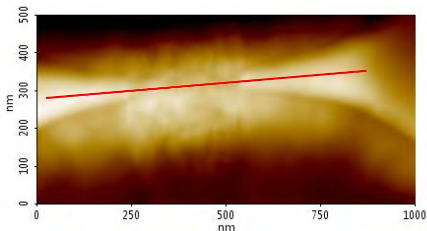
**FIGURE 1.** Contact mode AFM topography image of the first and properly fabricated vacuum-channel device's (Device 4) sensor-drain interface, vacuum-channel, and insulated gates region. The overlaid red line corresponds to the topography line profile displayed in Figure 2. Scan size: 500 x 1000 nm, image size: 380 x 190 px.
