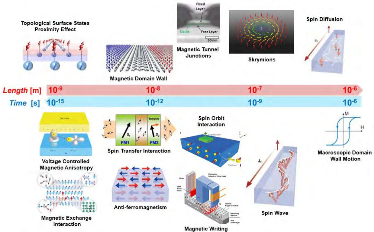
FIGURE 1. Various fundamental spin interaction mechanisms and spintronic devices in time and length scales. Revised from [3].
