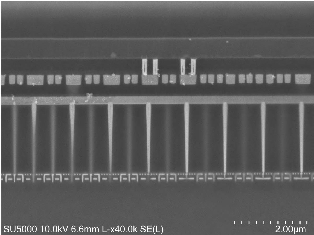
**FIGURE 2.** Higher Magnification of Cross Section of stacked chips Prepared with a pico-second laser tool and Broad Argon ION Beam Tool.
