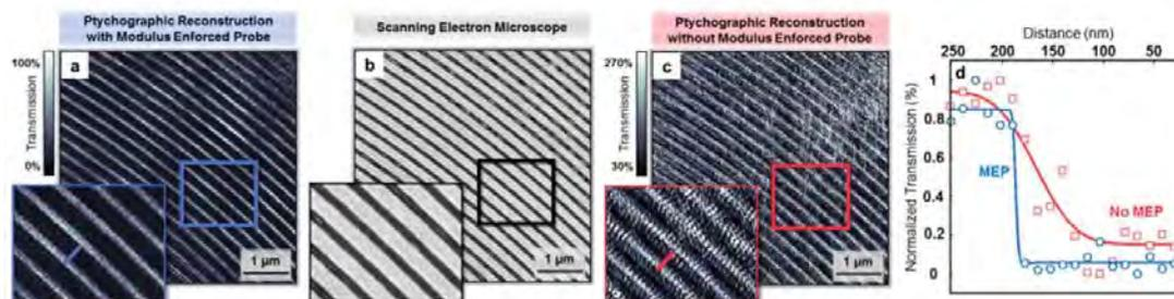
**FIGURE 1.** Ptychography CDI transmission image (a) reconstructed using the MEP technique, compared with an SEM image (b) and ptychography reconstruction obtained without the MEP technique (c). Lineouts (d) show 12.6nm resolution for the MEP reconstruction.
