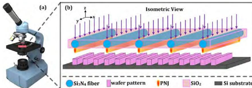
**FIGURE 1.** (a) Illustrated diagram showing a coherent optical microscope and (b) the mechanism of microfiber array-assisted CD metrology.
