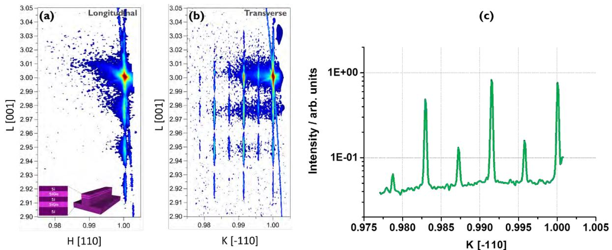
**FIGURE 3.** Reciprocal space maps (RSM) in the vicinity of the asymmetric (113) reflection acquired on 16nm wide fins in (a) longitudinal and (b) transverse direction. (c) Section along *K* through the transverse RSM averaged over *L* (2.91 - 2.99).
