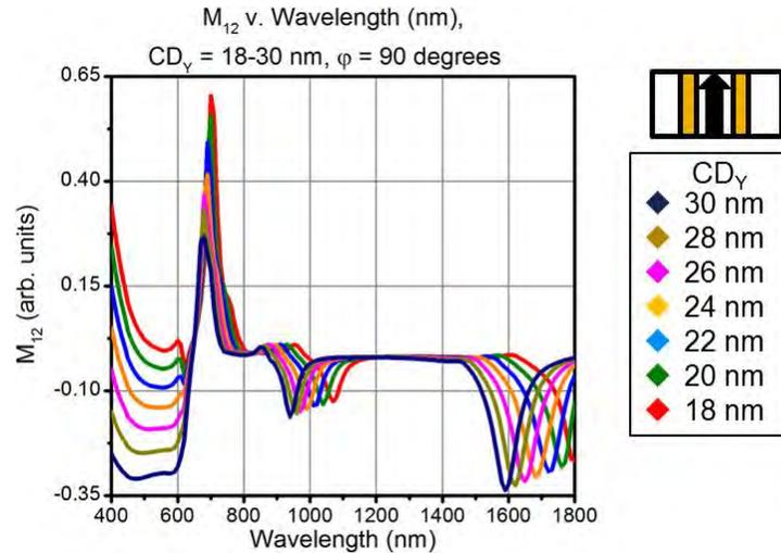
**FIGURE 5.** The M12 Mueller Matrix element for a copper cross-grating Structure for a CD values between 18 nm and 30 nm for the thin metal lines in the cross-grating.[5, 6]
