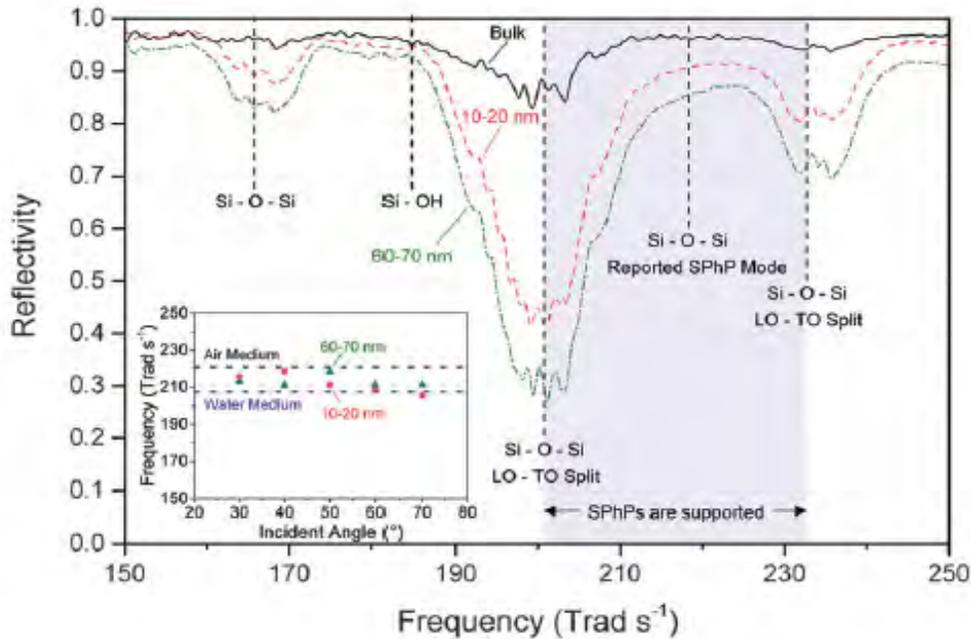
**FIGURE 1.** FTIR-ATR reflectivity of packed beds of 10-20 nm and 60-70 nm diameter  $\text{SiO}_2$  nanoparticles, and a bulk  $\text{SiO}_2$  film, vs frequency at an incident angle  $70^\circ$
