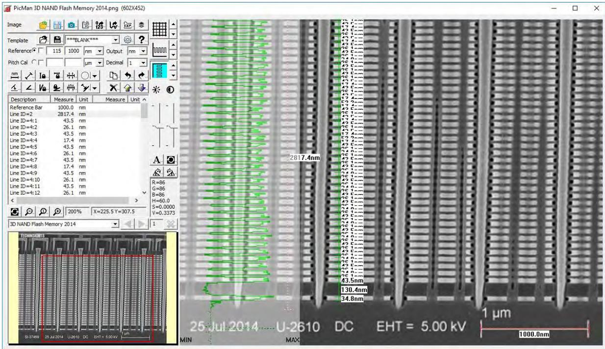
FIGURE 2. Cross section of a 3D V-NAND device (low magnification image). [2]
