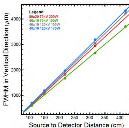
**FIGURE 2.** The x-ray beam size vs. the source to detector distance for a variety of electron beam configurations, from which the beam divergence was determined.
