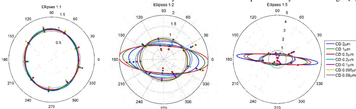
**FIGURE 3** Polar plot of the normalized Rapid Nano signal for nine separate detection angles from Au ellipses of varying aspect ratios, for a number of different critical dimensions.
