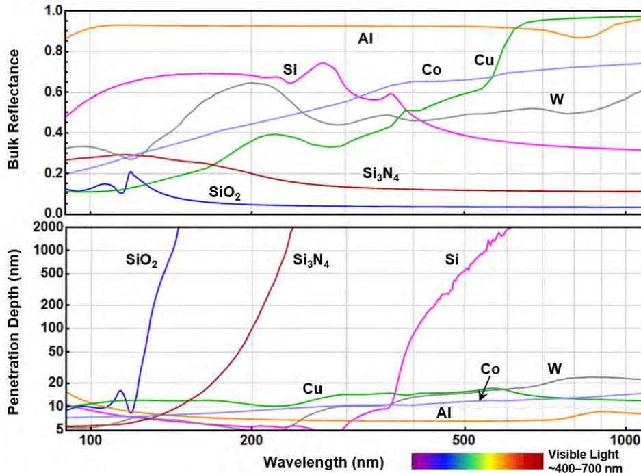
**FIGURE 1.** Reflectance and penetration depth for some materials common in semiconductor manufacturing. Note logarithmic scale for wavelength and penetration depth.
