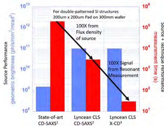
**FIGURE 3.** Comparison of raw source performance (left axis) and CD measurement time (right axis) for a 200um x 200um measurement pad on a 300mm wafer.
