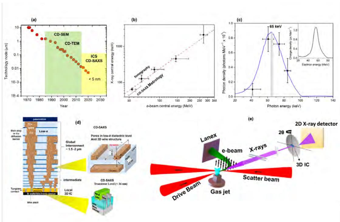
**FIGURE 1.** (a) Technology node versus year, indicating era of CD-SEM and future era of ICS CD-SAXS, (b) X-ray energy versus electron beam-energy [4, 6] (c) X-ray beam profile [4, 6] displaying the 65 keV band, (d) Various CD-SAXS and 3D tomography metrology applications in the integrated circuit, and (e) schematic layout of Inverse Compton scattering CD-SAXS beamline
