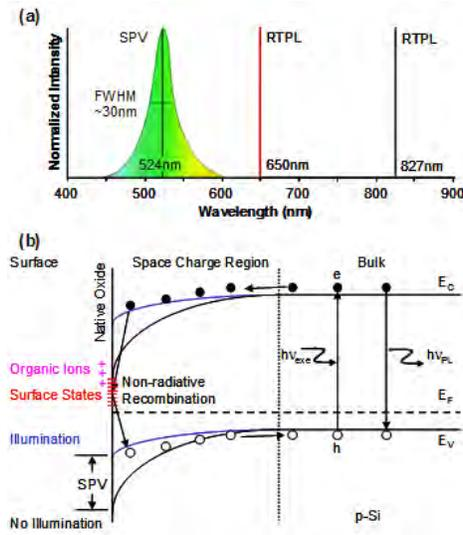
**FIGURE 2.** (a) spectral distribution of excitation light source and (b) schematic illustration of band bending with and without illumination.
