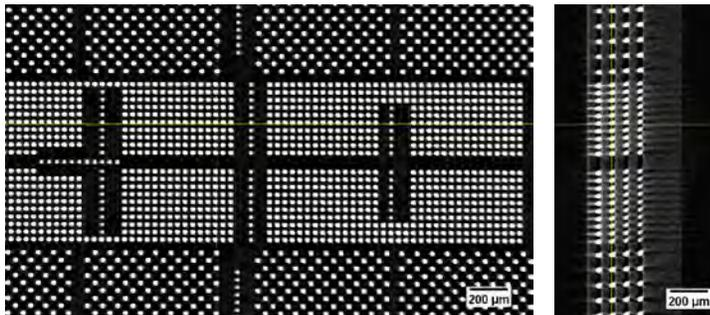
**FIGURE 1.** Two virtual 2D images (plane view and cross-section view) of a HBM stack, based on a 3D data set from micro X-ray tomography. Nondestructive imaging.
