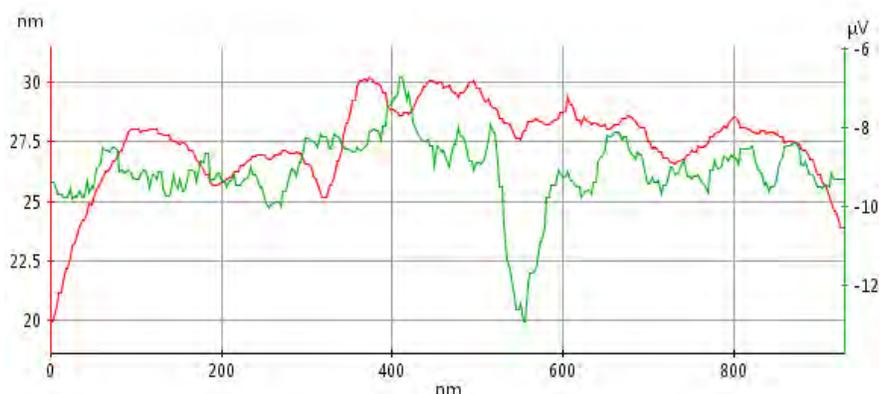
**FIGURE 5.** Line profiles of the AFM topography (red, left y-axis in nm) and the capacitance data (green, right y-axis in  $\mu\text{V}$ ) of the Device 6 area scanned in Figures 4 and 6.
