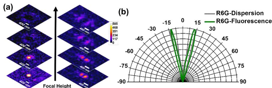
**FIGURE 2.** (a) Stacked fluorescence images taken at increasing focal plane height above the plasmonic grating. (Left) Angled SPCE and (Right) Airy disc pattern from the isotropic emission of a SM spreading with increasing focal height. Scale bar: 400 nm. Image exposure: 10 sec. (b) The normalized emission angle range for a SM of R6G plotted against the emission range predicted by the SPR dispersion and dye emission properties.
