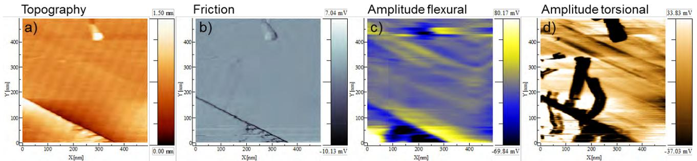
**FIGURE 2.**  $492 \times 492 \text{ nm}^2$  scanning probe images of the same area of a graphite sample displaying different signals. a) Topographic image taken at 280 nN applied normal (set-point) force; b) Friction (lateral force) signal image; c) Amplitude of the flexural response of the cantilever, demodulated at 1.65 MHz and d) amplitude of the torsional response of the cantilever, demodulated at 3.94 MHz. Dislocation system can only be distinguished at image d), by the dark lines.
