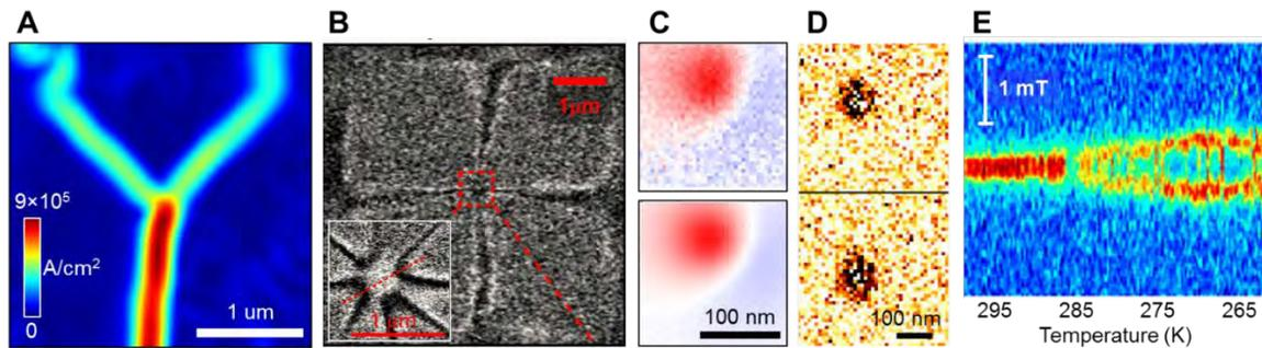
**FIGURE 2.** Examples of imaging nanomagnetism by NSDM: (A) Image of current density in a  $50 \times 50 \text{ nm}^2$  Pt nanowire [5], (B) Image of magnetic vortex in a 50 nm thin film of  $\text{Fe}_{20}\text{Ni}_{80}$  [6]. (C) Image of a single FeCo nanoparticle (experiment and simulation) [7]. (D) Image of magnetic noise from single superparamagnetic magnetite nanoparticles [9]. (E) Local field at a FeGe surface above and below the helimagnetic phase transition [9].
