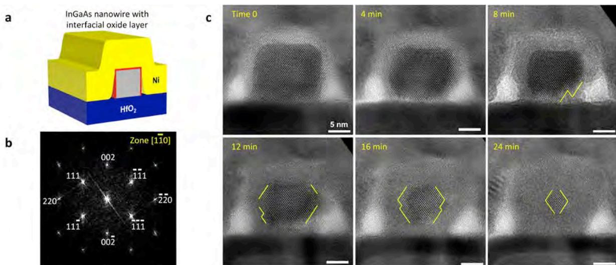
**FIGURE 2.** (a) schematic of Ni contacting with an InGaAs nanowire cross-section that sits on the  $\text{HfO}_2$  dielectric layer. (b) fast Fourier transform (FFT) image of the corresponding nanowire cross-section, showing the diffraction pattern along the zone axis
