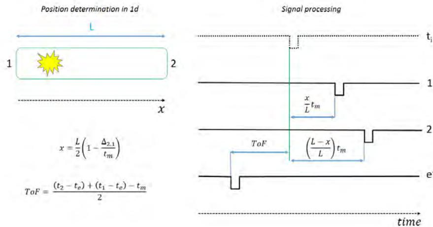
**FIGURE 1.** Position determination of ion hit in 1d case.  $t_i$  is the virtual signal denoting the real Time of Flight, channels 1 and 2 are two opposite outputs of meander wire.  $e^-$  is the electron start signal.  $t_m$  is the “meander time” associated with an imposed position dependent time delay on the actual ion arrival time.  $\Delta_{2,1}$  is the difference in time between signals on channel 2 and 1.
