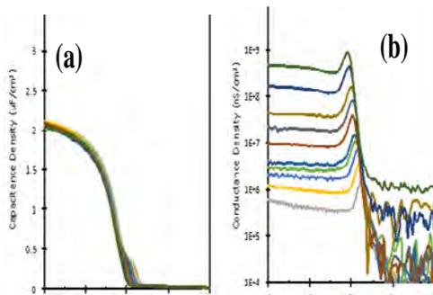
**Figure 3: Electrical Characterization of Al<sub>2</sub>O<sub>3</sub>-HfO<sub>2</sub> alloy / Si<sub>0.5</sub>Ge<sub>0.5</sub>(001)/Si(001).** (a) C-V shows  $D_{it} \sim 2 \times 10^{12} / \text{cm}^2\text{-eV}$  using the conductance method. (b) G-V shows low leakage. A Ni gate was thermally evaporated along with an Al back contact.
