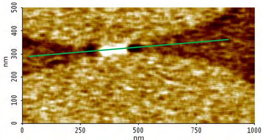
**FIGURE 3.** An SCM capacitance image of the region containing Device 4's sensor-drain interface, vacuum-channel, and insulated gates. Brighter colors correspond to relatively more positively charged areas on the device whereas darker colors correspond to relatively more negatively charged areas. The overlaid green line corresponds to the capacitance line profile displayed in Figure 2. Scan size: 500 x 1000 nm, image size: 380 x 190 px.
