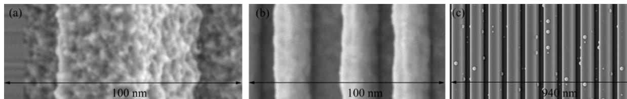
**FIGURE 2.** Simulated SEM images of 3 virtual samples. The samples were imaged with tilts at  $5^\circ$  increments from  $-85^\circ$  to  $85^\circ$  from the normal (axis of rotation along the lines). The views shown here are at  $20^\circ$ .
