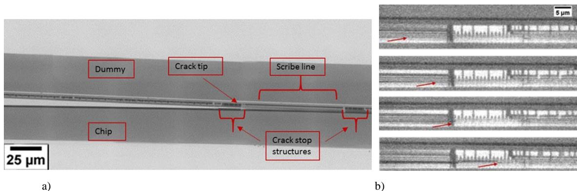
**FIGURE 3.** a) Stitched radiograph of a micro-DCB sample under load. The crack penetrates the crack stop structure from the chip side. The image is rotated clockwise by  $90^\circ$ , b) series of the virtual cross-sections based on nano-XCT, revealing the crack propagation at the Cu/low-k crack stop structure.
