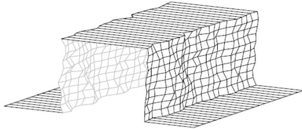
**FIGURE 2.** A randomly generated rough line of which a small section is shown here. At first, a flat line with a length of 2  $\mu\text{m}$ , width of 32 nm and a height of 32nm is constructed. The sidewalls of the flat line are replaced with randomly generated rough surfaces. Note that the top of the line and the substrate, on which the line is located, remains flat.
