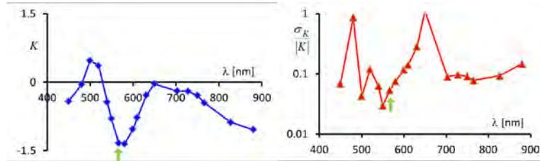
**FIGURE 3.** The left graph shows a measured  $K$  as function of  $\lambda$  on a product wafer and the right graph shows the normalized  $1\text{-}\sigma$  variation of  $K$  across the wafer. The arrow indicates a wavelength with a high  $K$  and low  $\sigma_K/K$
