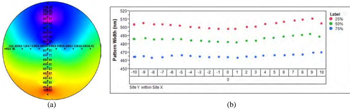
FIGURE 3. (a) Wafer map of pattern width at heights of 75% from bottom and (b) their value changes, measured at heights of 25, 50 and 75% on Y axis of wafer
