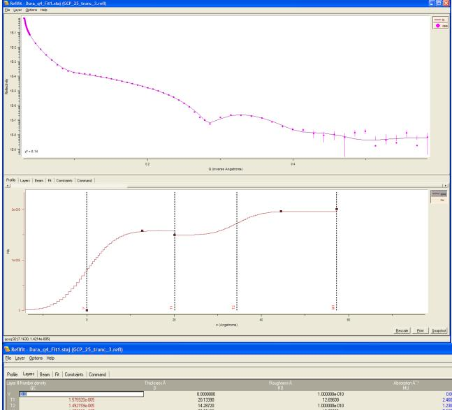
The target thickness for the 5.22% solution was 50 Å, but this XR fit indicates a total thickness for the PPR of ~34 Å. We extended the analysis for this sample, using NR in a dry environment and in a 90% RH (D<sub>2</sub>O) environment. This was the sample that we put Nafion on for additional NR measurements. (Thanks to Joe Dura for completing this data fit.)
