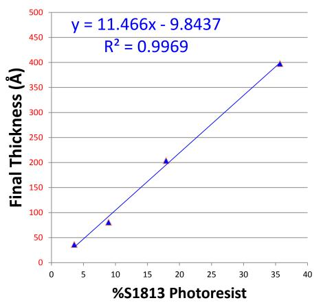
By entering the target thicknesses of 30 Å and 50 Å into the best fit equation, we determine S1813 concentrations of 3.47% and 5.22%.
