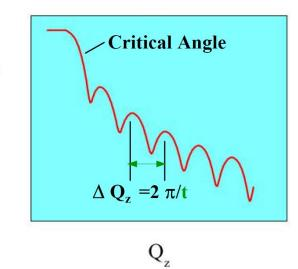
• Specular Reflectometry measures Reflected Intensity vs. grazing angle  $\theta$  or  $Q_z$  with  $\theta_i = \theta_f$  $Q_z = 4\pi \sin \Theta / \lambda$
