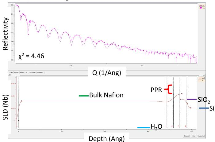
H<sub>2</sub>O vapor reveals a strong dip in sld between Nafion and the PPR layer, corresponding to a single water-rich layer at the interface
