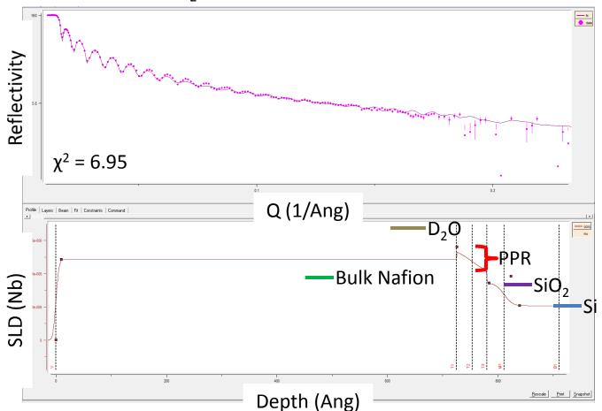
$D_2O$  reveals a strong peak in sld between the Nafion and PPR layers, also corresponding to a single water-rich layer at the interface
