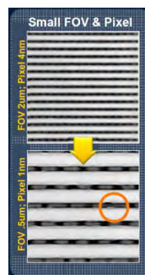
FIGURE 2. Improvement in defect detection by increase of pixel resolution (source: Applied Materials)
