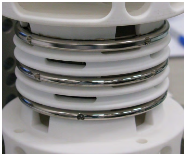
FIGURE 4. Electron mirror with the three electrodes on variable potential. The fourth electrode is hidden inside the lower insulator.
