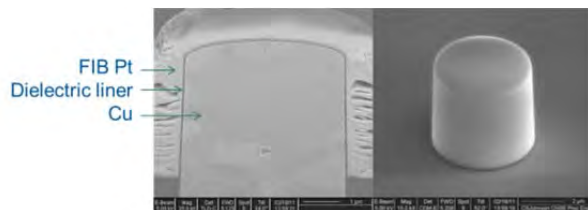
FIGURE 1. A Focused ion beam (FIB)/SEM image (left) shows a revealed TSV; tilt SEM image (right) shows a smooth Si surface.
