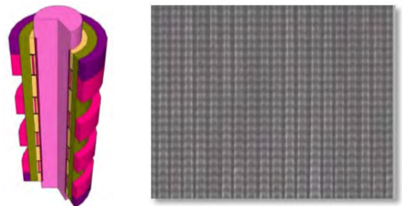
Figure 2: Vertical NAND (3-D) Structure Schematic
