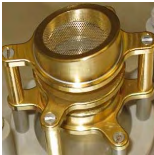
FIGURE 5. Grids for generating the retarding electric field in the spectrometer.
