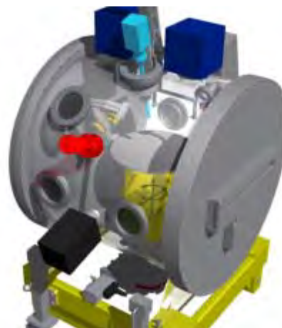
FIGURE 2. CAD model of the analytical platform for 450 mm wafers (design study)
