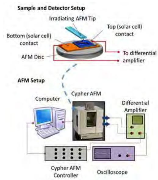
FIGURE 1: Experimental setup for X-ray AFM probe and Cypher AFM system coupled to differential amplifier and computer.
