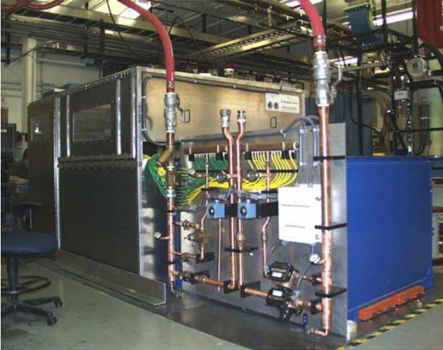
20 KHz, 10 MW Polyphase Pulsed Converter
