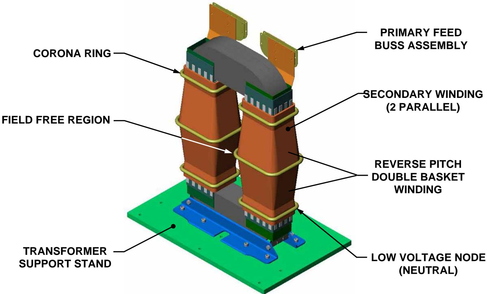
*Advanced Winding Topology Minimizes Field Stresses And Leakage Inductance*
