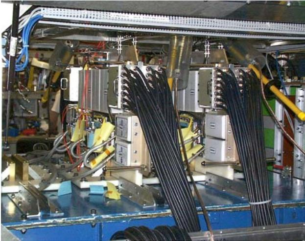
20 KHz IGBT Switching Assemblies
