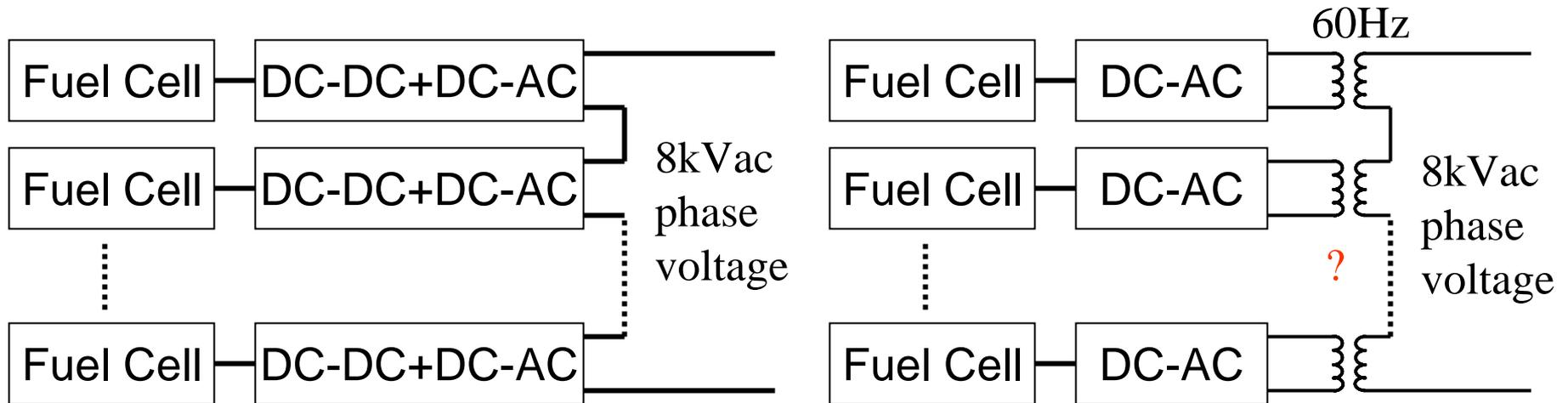
Two options to avoid high common mode voltage on upper level fuel cells
