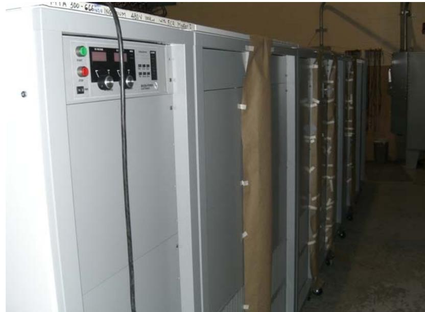
Photograph: a 400-kW current source DC-DC converter
