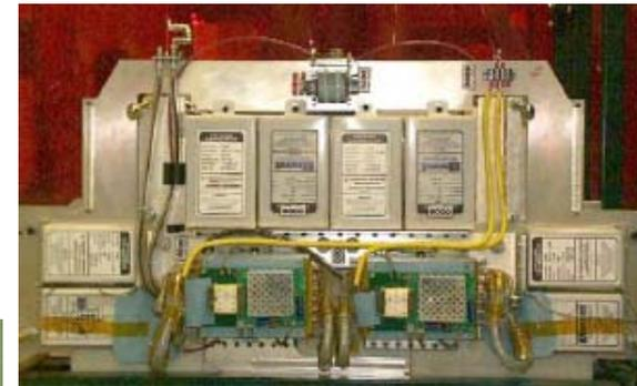
IGBT switch plate assembly
