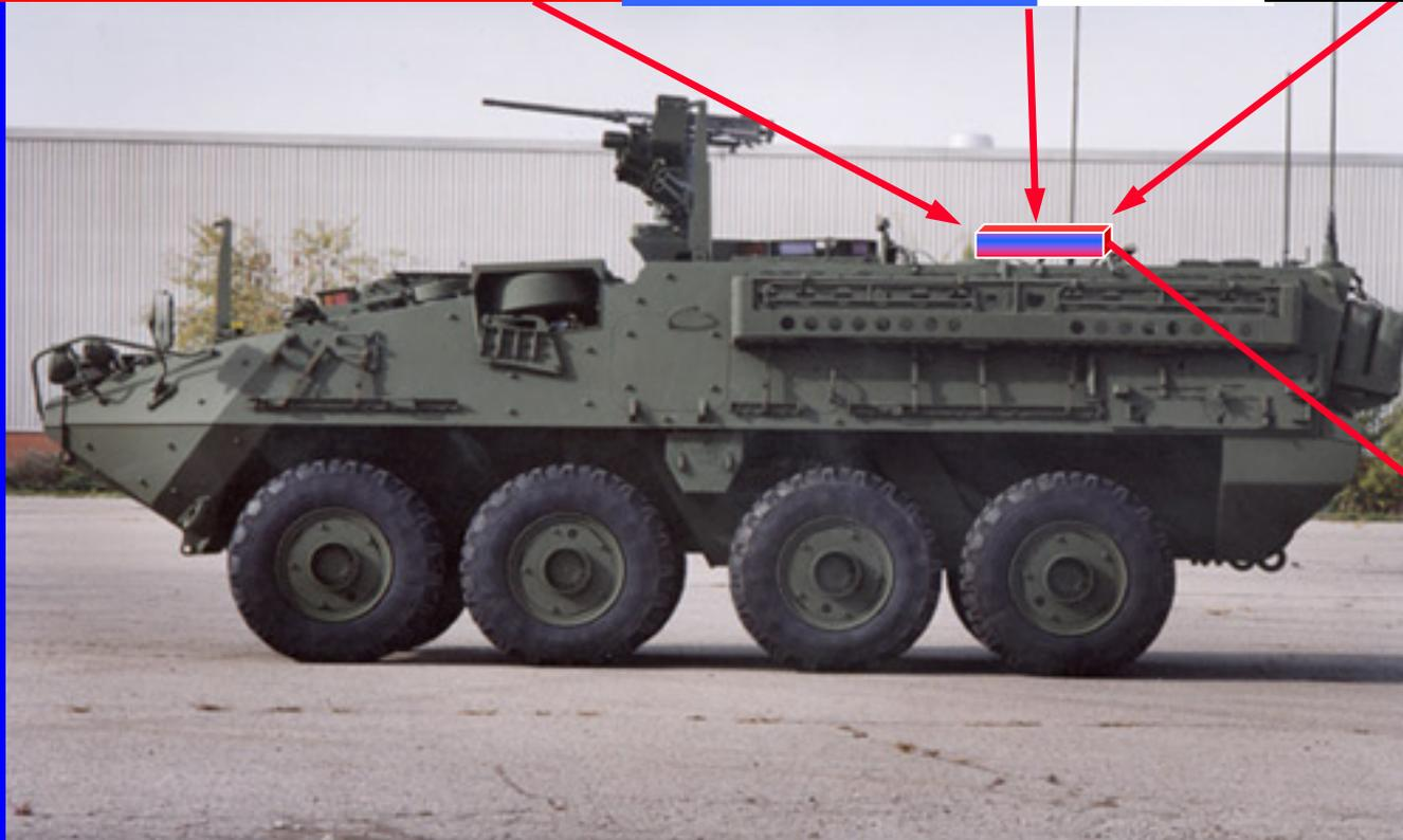
Current Prototype System is located behind turret and in front of the rear hatch ports of egress. System also includes on-board water storage vessel.
