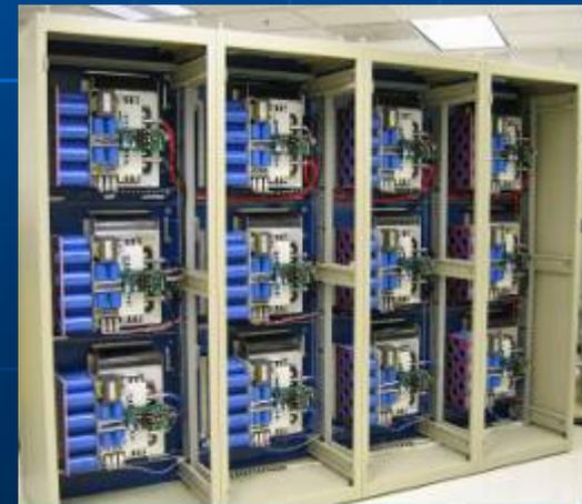
Cascade multilevel inverter
