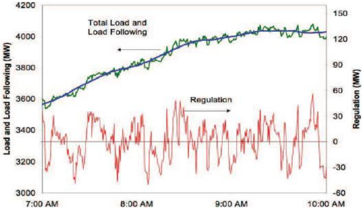
**Regulation is near zero-energy service compensation for minute-to-minute fluctuations in total system load and uncontrolled generation**
