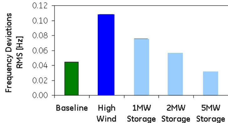
5MW of "fast" energy storage resulted in similar frequency performance as the baseline scenario; near-term potential project
