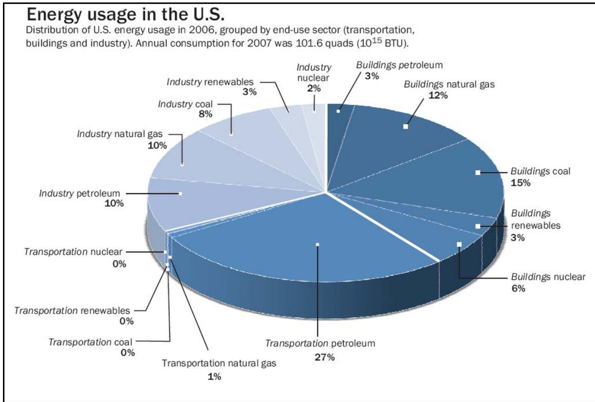
**Figure 2.** Energy usage in the U.S. This chart shows a detailed breakdown of energy usage by sector in the United States in 2006. According to the chart, the largest consumers of energy in the United States are commercial and residential buildings and transportation. (Richter, p. S21)
