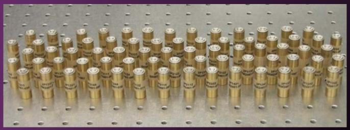
SRM Casings made from electroform process
