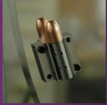
Standard Bullets manufactured using a numerically controlled diamond turning operation
