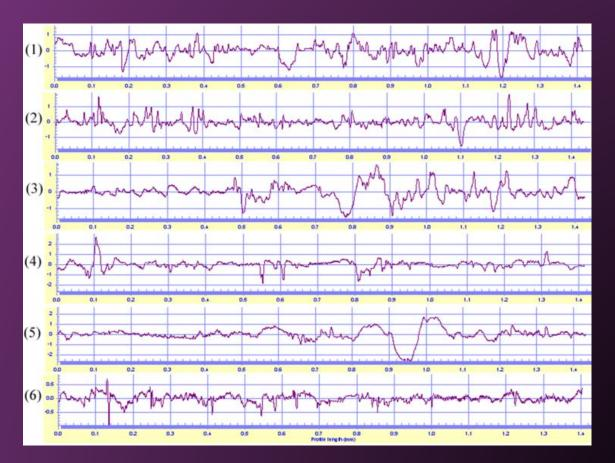
Surface Profile measurements from the six lands on the Standard Bullet (after digital Gaussian filtering and curvature removal)
