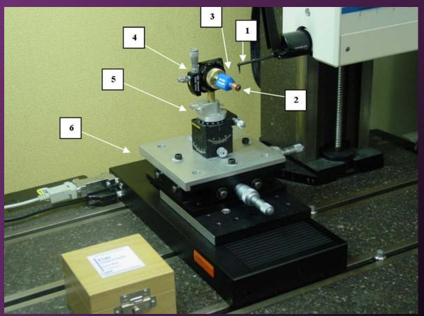
Measurement setup for NIST bullet signature measurement system: 1) Diamond stylus; 2) Standard bullet; 3) Bullet holder; 4) Rotary stage; 5) Horizontal rotary stage; 6) X-Y stage.
