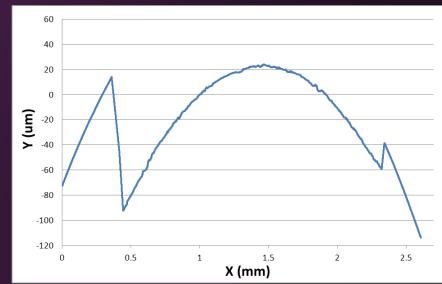
Stylus profilometer measurements of master bullets result in digital profiles of bullet LEA's
