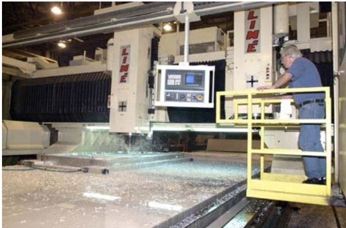
Figure 2 Machining a large aerospace cargo floor
