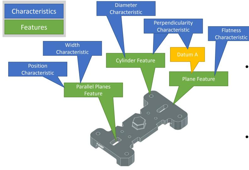
The fundamental constructs behind QIF: Features & Characteristics
