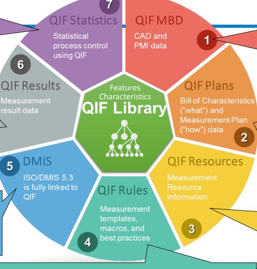
Create measurement rule templates. (e.g., *If a Surface Profile tolerance value is less than* **x**, *then use a CMM method with at least* **y** *number of point/sq.in.*)
