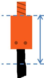
This distance (for simplicity I'm calling it the sample) **should be 40mm**. It can be made to fit so long as it's greater than 28mm as described above. In all cases, be careful that the sample doesn't hit the bottom of the can (there is 65mm space below beam center.)
