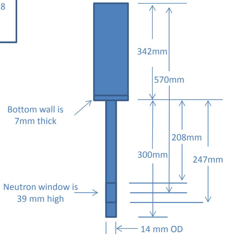
For using with ICEoxford OC/HFBS OC, the distance between the top flange to beam center is 1305mm, plus 4mm Oring =1309mm. With the 15T DR's flange on the very top position, after mounting the cylindrical IVC, the distance between the bottom of the flange and the center of the neutron window is 1310 mm. Perfect fit!
