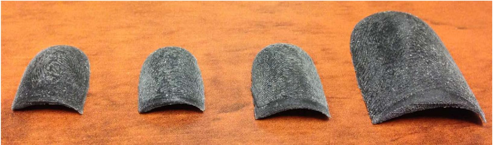
**Fabricated 3D synthetic artifacts of different finger sizes and hardness**
