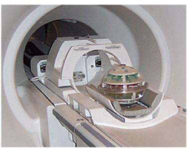
"Phannie", a phantom to calibrate MRI machines developed at NIST http://www.nist.gov/pml/electromagnetics/phanni e 051110.cfm
