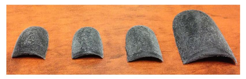
Fabricated 3D synthetic artifacts of different finger sizes and hardness
