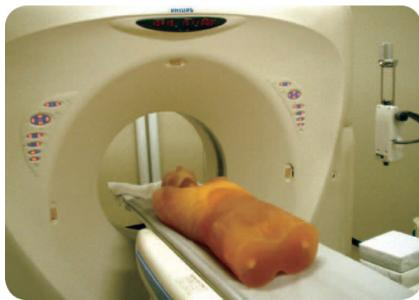
Torso Phantom to calibrate CT Scan machines https://www.kyotokagaku.com/products/detail03/ph-4.html
