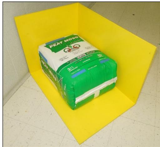
**Figure 3-1. Dimensional Measuring Frame.**
