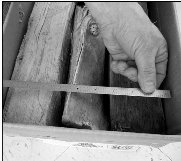
6. Individual Piece Length. Remove the wood from the package and measure the length of each piece of wood (see Table 3-5. “Minimum Number of Pieces to be Measured for Length”). If the piece of wood is uniform in shape, take at least one point-to-point measurement along the center line of the longitudinal axis (see Table 3-6. “Determining Piece Length, (a) Uniform Shapes” for examples) and record the value.
