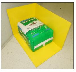
Figure 3-1. Dimensional Measuring Frame
