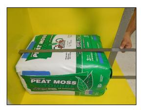
Figure 3-5. The packaging tail on the end of the package can affect this measurement so it has been folded over and taped against the end of the package.
