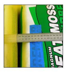
Figure 3-3. The rigid frame allows the observer to hold the zero reference point firmly in place.
