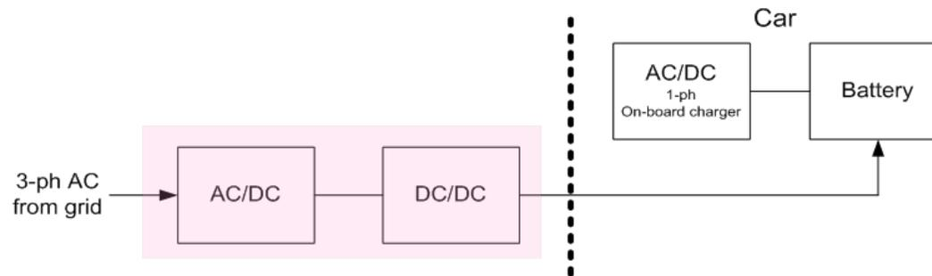
Fast charging system for a car battery
