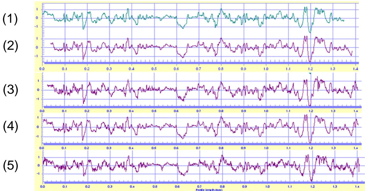
Measurement comparison of four techniques tracing the same SRM bullet:
