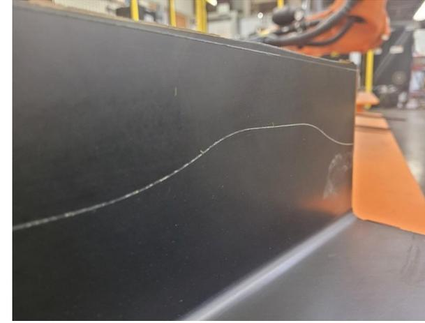
CFRP part with Scribe Line
