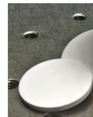
Sintered Al<sub>2</sub>O<sub>3</sub> discs of SRM 1976b
