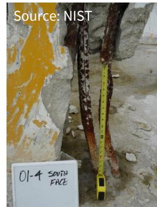
5 Short, high lap splices in columns
