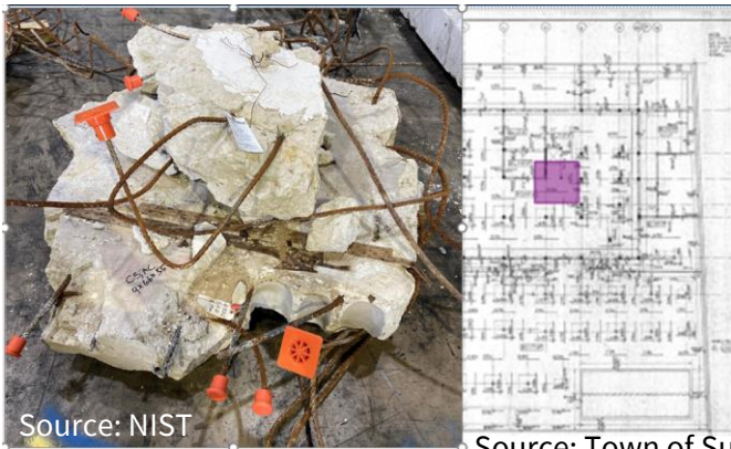
2 Placement of Top Bars in Column Strips
