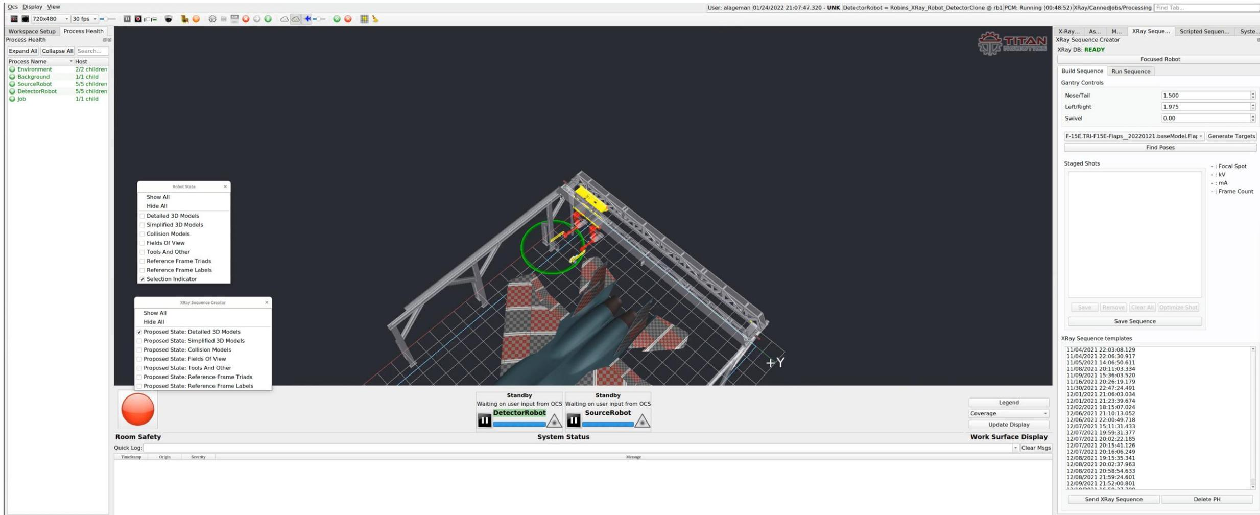
The screenshot displays the X-Ray Sequence Creator software interface. The main window shows a 3D model of a robot arm with a green circle highlighting a specific area. The interface includes several panels and controls:
