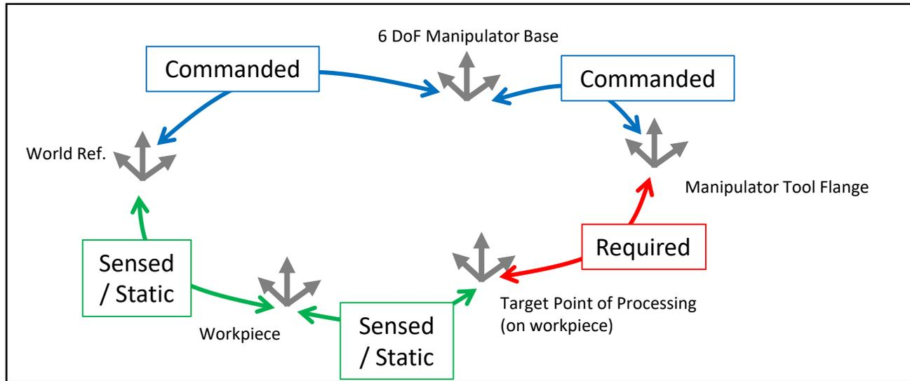
When designing a system, we are iterating on the choices of Process Tooling, Manipulator Hardware Selection, and Workpiece Localization Approach to create a positioning uncertainty stack such that is less than the allowable uncertainty of the Process and allowed by the capabilities of the Process Tooling.
