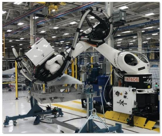
LARGE Cartesian volume, minimal orientation change, minimal joint range, INCREASED accuracy
