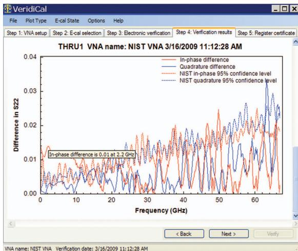
**Figure 4.** NIST's VeridiCal software compares the differences between your calibrated measurements and traceable NIST measurements of the states of the electronic calibration unit to the NIST uncertainties.
