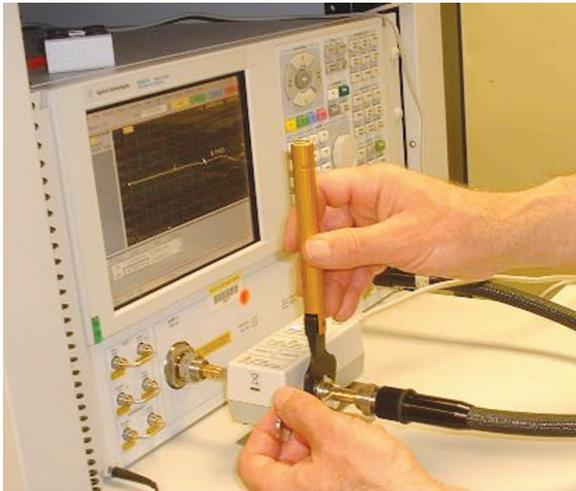
**Figure 1.** A single connection of the electronic verification unit to the vector network analyzer is all that is required to accomplish the verification process. Once the electronic calibration unit is connected, all of the measurements and analysis are performed automatically.
