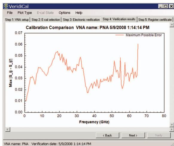
**Figure 2.** This calibration comparison metric is the first thing shown after running NIST's VeridiCal software. It provides a bound on the differences of measurements corrected by your VNA calibration and measurements corrected by a traceable NIST calibration. See "NIST Metric for Calibration Accuracy" for more on the meaning of this metric.
