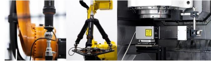
Single and triple ballbar systems, and multi-axis laser calibrator (Renishaw)
