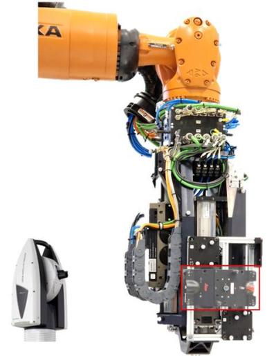
Leica AT960 laser tracker and drilling end effector with mounted T-Mac (highlighted)
