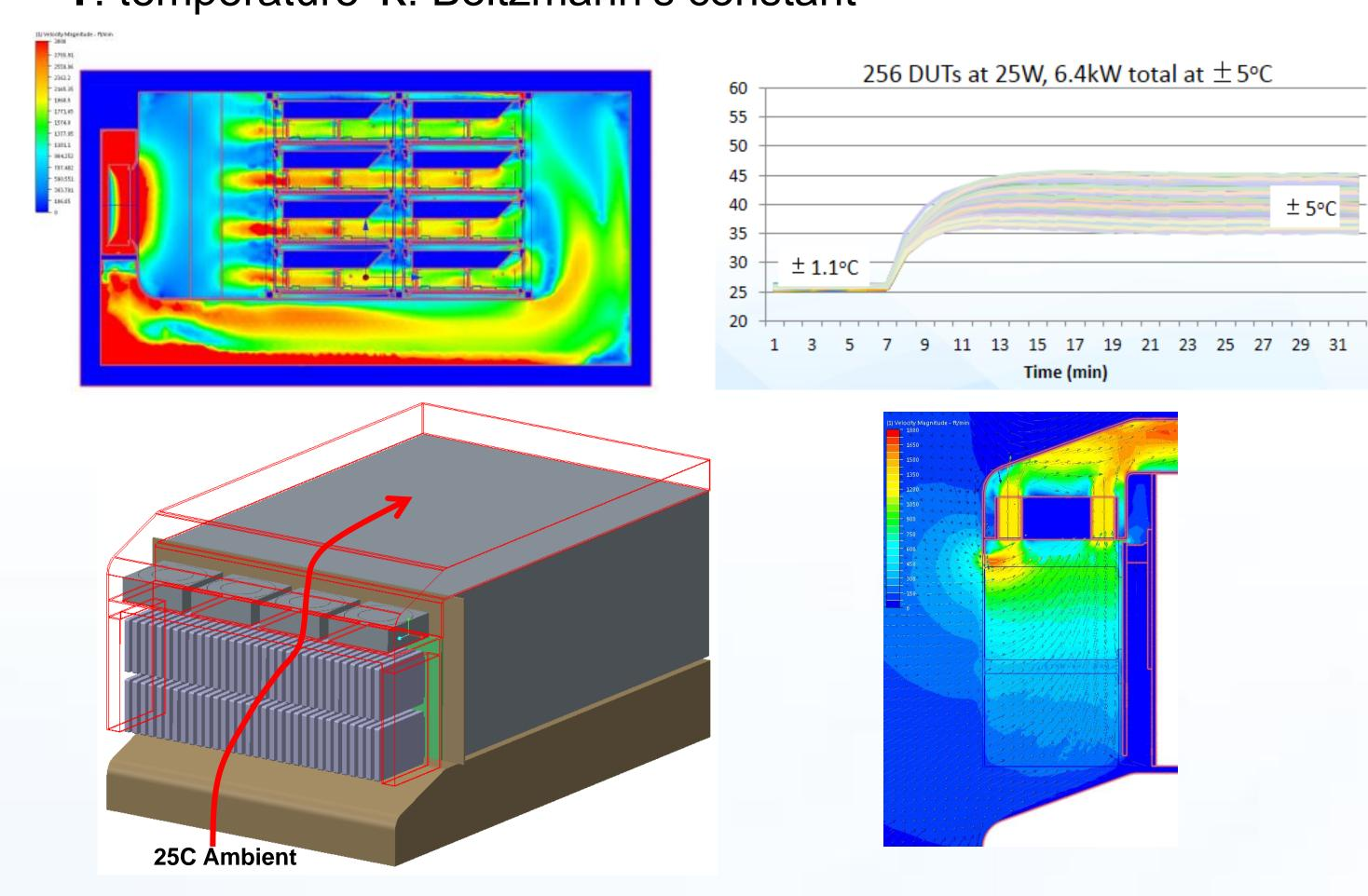
Active Cooling for Endurance, Closed-loop Ambient for Production
