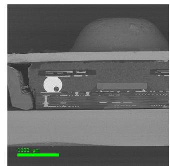
**Figure 6.** Low-magnification backscattered electron (BSE) image of a mobile phone home button after the workflow described in Figure 1. The cross-section is shown mounted on an Ilion II blade. The complete device was cross-sectioned 6 x 1.4 mm (L x D) thick in the microPREP system in 45 min. The Ilion II system's cross-sectional area is  $\sim 2$  x 1.4 mm.
