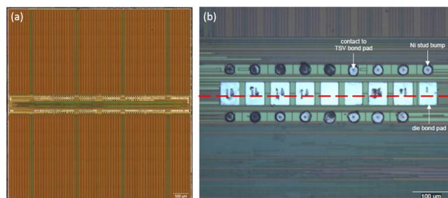
**Figure 4.** Optical microscope images of K4A4G085WD memory die; (a) low magnification image; (b) close-up to show the TSV bond pad.
