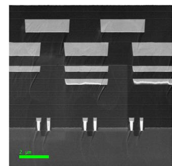
**Figure 7.** BSE image of the transistor structure in the mobile phone home button. This region is  $\sim 600$   $\mu\text{m}$  below the ceramic and resin layers and  $\sim 600$   $\mu\text{m}$  above the metal base of the button. Both cut with the workflow described in Figure 1.
