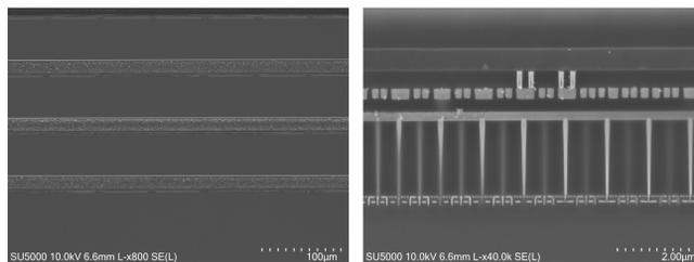
**Figure 3.** SEM images of cross-section of stacked chips prepared with microPREP system and then broad Ar ion beam tool at low and high magnification.
