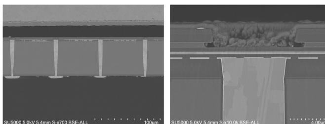
**Figure 5.** SEM images to show an array of TSVs and the details of an individual TSV. Grain structure can be clearly observed.
