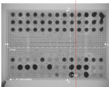
**Figure 2.** X-ray image of the K4AAG045WD-4CRB package with cross-section location highlighted by the red line.
