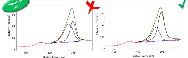
N1s industrial XPS spectra, with a free fit (left) and a constrained fit based on the pARXPS and the Nano-ARPES measurements (right).
