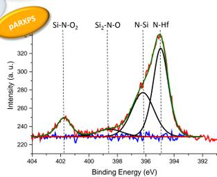
N1s pARXPS spectra and fitted peaks of the HfON/SiON/Si stack obtained at 23.75°.
