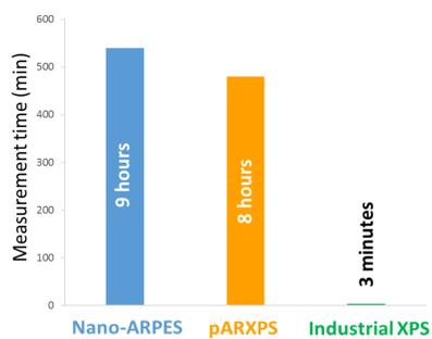
Time of acquisition per point of the three systems to obtain the different spectra of the HfON/SiON/Si sample.
