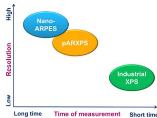
Comparison of the three XPS capabilities based on resolution and time of measurement.
