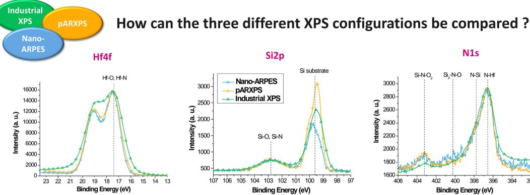
Comparison of Hf4f, Si2p and N1s XPS spectra obtained by Nano-ARPES, pARXPS and industrial XPS on the HfON/SiON/Si industrial gate stack.
