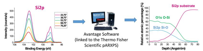
Chemical profile reconstruction obtained by applying the maximum entropy concept to the angular information (Nano-ARPES and pARXPS).
