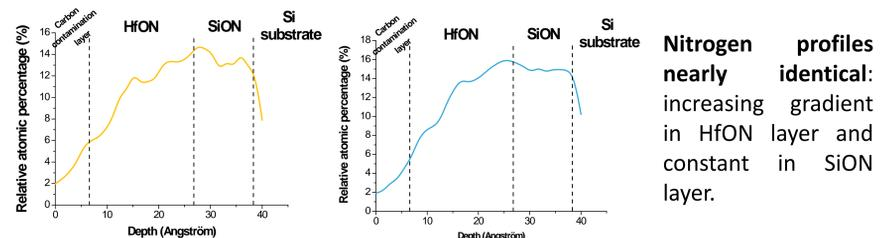
Nitrogen distributions obtained by chemical profile reconstruction with pARXPS spectra (left) and Nano-ARPES spectra (right).
