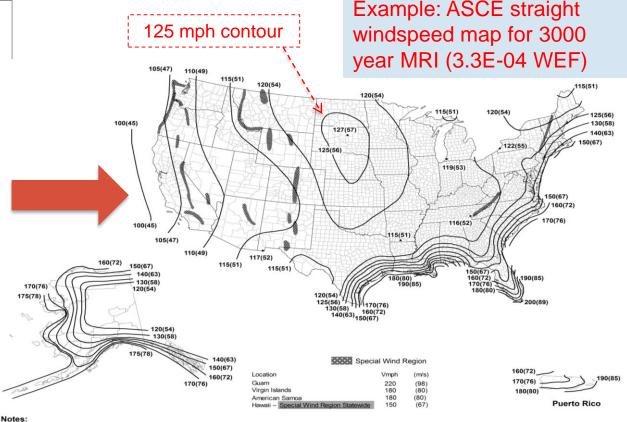
1. Values are nominal design 3-second gust wind speeds in miles per hour (m/s) at 33 ft (10m) above ground for Exposure C category.
