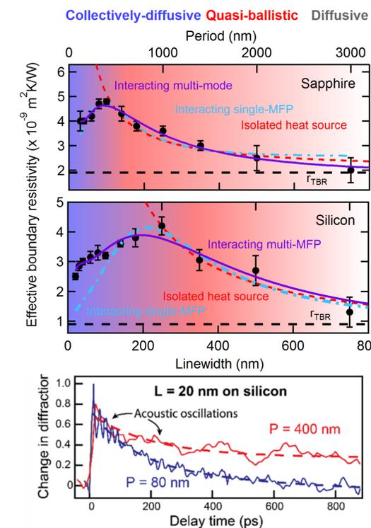
Probing heat dissipation away from heat sources as small as 20 nm in linewidth, we confirmed period-dependent non-diffusive transport, where closely-spaced nanowires cool faster than widely-spaced ones.
