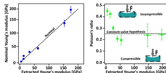
New trend in Poisson's ratio is observed in SiC:H films: Increasing hydrogenation decreases the network connectivity below critical value  $\sim 2.5$ . The material then transitions from compressible to incompressible.
