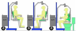
Figure 4 – Graphic showing the concept of placing a patient onto a toilet or chair with the HLPR Chair. The patient drives to the target seat (left), manually rotates near or over the seat (middle) while the torso lifts support the patient and the seat retracts, and then is lowered onto the seat - toilet, chair or bed (right)
