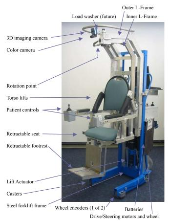
Figure 1 – Photograph of the HLPR Chair prototype.
