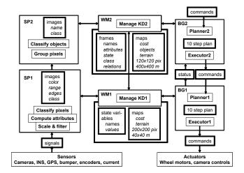
Figure 7 – NIST 4D/RCS 2-level, hierarchical control architecture developed for the DARPA LAGR Project and planned for implementation on the HLPR Chair.
