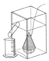
Figure 3-1. Example of a Displacement Vessel
