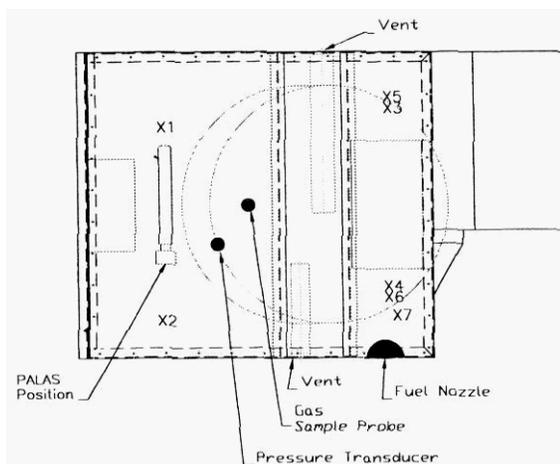
Figure 2a. F-22 Wheel Well Dry Bay Simulator: Plan View.
