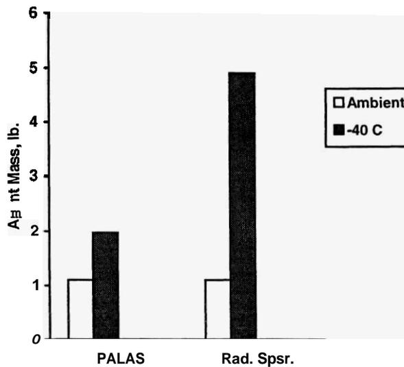
Figure 4. Comparison of **PALAS** and Conventional Suppressor in DBFS Tests (24.6 ft<sup>3</sup> volume) bay fires during previous live-fire tests [10]. A conventional Halon 1301 bottle for the 24.6 ft<sup>3</sup> volume dry bay would contain 1.3 lbs of agent, based on a 9% v/v concentration at the lowest expected temperature of -65 °F [11]. Estimated values of agent mass and volume are presented in Table 5 for a Halon 1301 system, PALAS, and the radial suppressor.
