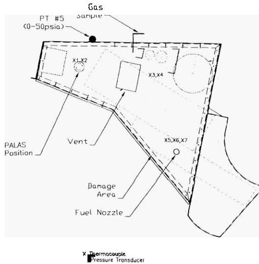
Figure 2b. F-22 Wheel Well Dry Bay Simulator: Side View.
