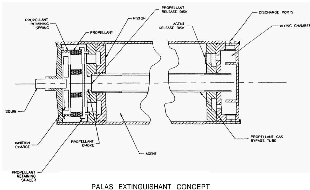
Figure 1. Schematic Representation of PALAS Unit.
