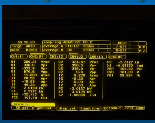
Discharging Test Data at 3kW
