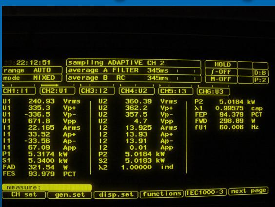
Charging Test Data at 5kW
