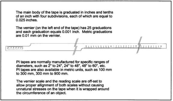
As the tape is wrapped around the circumference of an object, the reading portion of the tape and the vernier come into alignment. The smallest graduation on the main body equals 0.5 mm (0.025 in). The line on the
