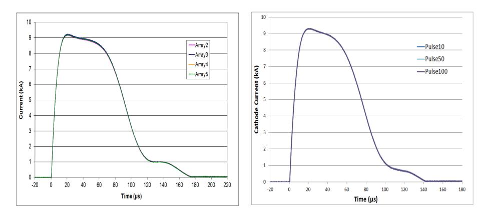
Four SGTO arrays (2 cm<sup>2</sup> die area) each switched at 9 kA Array #3 (2 cm<sup>2</sup> die area) Initially switched at 9 kA for 100 pulses
