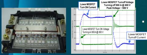
1200 V / 900 A Module Operating at 80°C Heat Sink Under Stall-Zero Condition for 200 hours
