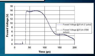
SiC SGTO module forward voltage drop Overlay of pulse 1 and 1000.
