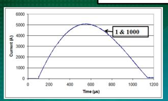
SiC SGTO module peak current. Overlay of pulse 1 and 1000.
