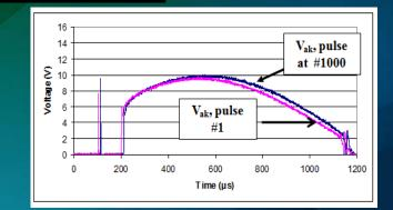
SiC SGTO module forward voltage drop. Overlay of pulse 1 and 1000.
