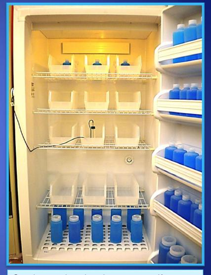
Continue using data logger to verify target set point temperature (4 to 6 °C) during weekly data download and make adjustments when needed
