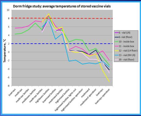
In the NIST vaccine refrigerator study, the dormitory-style unit exhibited severe temperature control and stability issues. Within 2 weeks of use, the refrigerator set point had drifted approximately 5 °C colder, freezing the vaccines contained inside.
