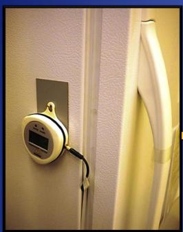
Attach logger display to outside of refrigerator
