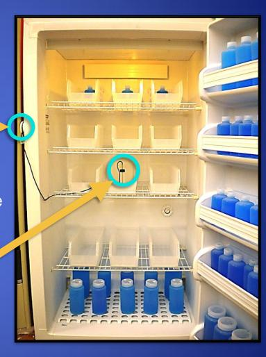
Place logger probe and bottle setup in a tray in the center of the refrigerator. Fix bottle in place with tape or Velcro.
