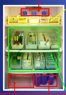
No storage in crisper drawers: thermally isolated + floor level runs cold. Remove drawers, fill space with water bottles
