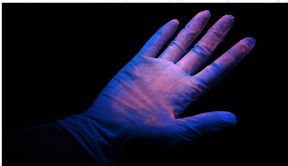
A NIST research scientist uses a fluorescently-tagged simulant to help screeners visualize typical trace residue contamination on gloves after handling explosives.
