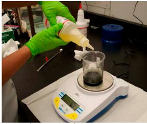
Mixing polyurethane with dye, and vacuum-degas
