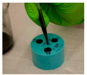
Use a dropper to fill mold with urethane. Vacuum-degas and let cure
