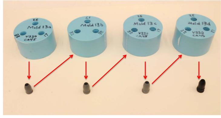
Master Bullet #'s 17, 32, & 38 used to create first mold (13a)
