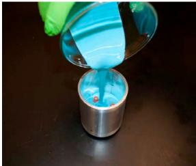
Pouring silicone into replication rig
