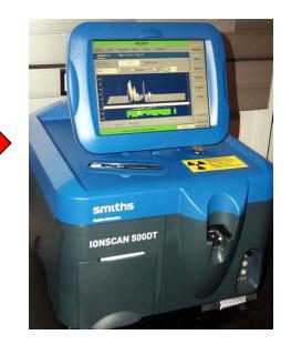
Most commercial explosive trace detectors (ETDs) can detect in the low nanogram range (a single crystal much smaller than the width of a human hair!)
