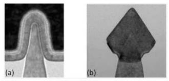
TEM images of Intel 22-nm PMOS tri-gate transistor (a) and
