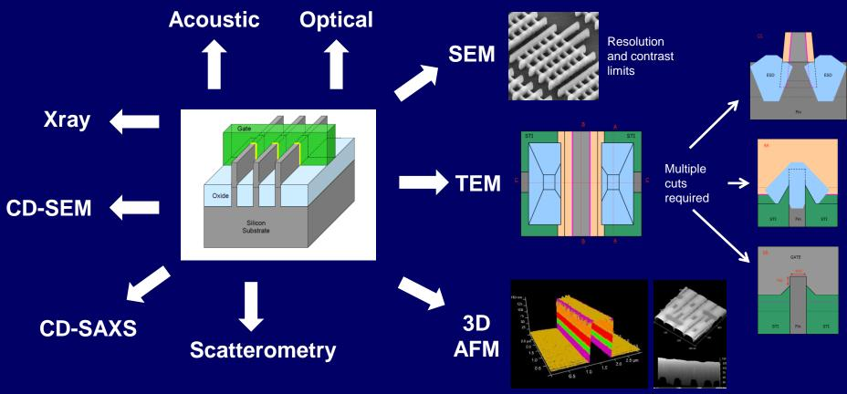
New capabilities to enable critical 3D measurements
