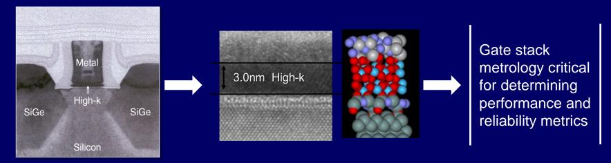
Introduction of HK/MG film stack increased need for accurate/precise measurement and control of ultrathin film composition and interactions; including <1nm films and interfaces</p>
