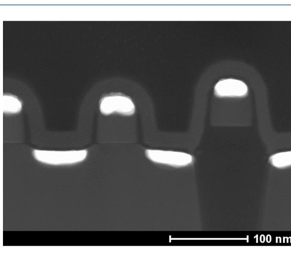
The STEM above shows a row of partially processed NMOS transistors. We see NiSi, but we do not see tungsten contacts. This is so we can analyze the surface roughness and coverage of NiSi, without the tungsten confounding the tomography. In the opaque reconstruction, below image "a", we see a rough NiSi surface, however, very uniform coverage. The semitransparent reconstruction, below image "b", is less informative, but
