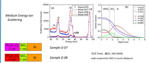
Comparison of the layer thickness measurements for the samples D07 and D08 using different analytical techniques. Results are given for two different densities of the silicate layers.
