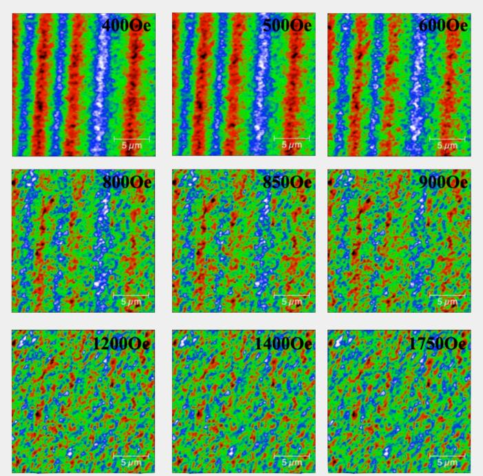
Stripe contrast starts to disappear with increasing in-plane magnetic fields, indicating that the magnetic bit profile is progressively destroyed.
