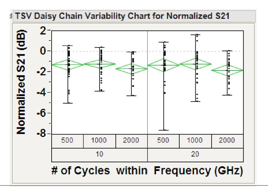
• The normalized graph show similar trend as previous graph. At 10 and 20 GHz, no main appreciable difference in RF signal characteristics between
