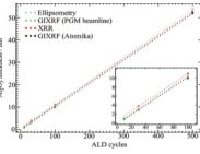
A complementary analysis of Al<sub>2</sub>O<sub>3</sub> layers on silicon with varying thicknesses is shown in the figure. The determined grazing incidence X-ray fluorescence and ellipsometry are in accordance with each other, which demonstrates the success of the complementary analysis.
