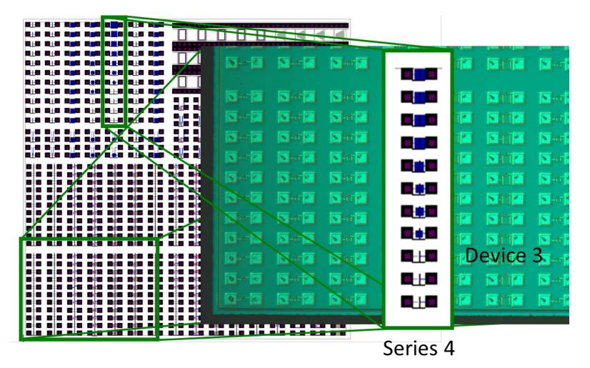
Target for probe based CBCM will be a test chip with a large variety of MOS capacitors from 0.1 to 100 fF.
