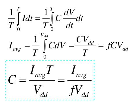
Q=Charge C=Capacitance V=Voltage I=Current t=Time T=Period f=Frequency
