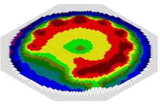
Film thickness map of a 2 nm SiON film with 9% nitrogen
