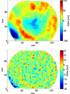
Flatness (top) and Nanotopography (bottom) of a polished Si wafer
