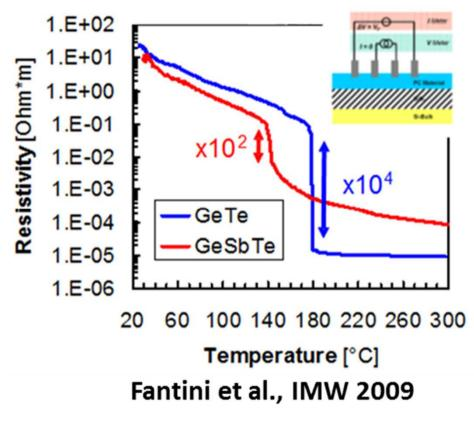
**Tx: Crystallization temperature** Tm: Melting temperature of crystal
